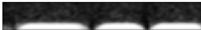
Figure 3.48: Blurred version of figure 3.47 using a Gaussian filter with a standard deviation of 1 pixel.
