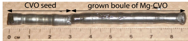
Figure 4.2: As-grown crystal of (\text{Co}_{1-x}\text{Mg}_x)_3\text{V}_2\text{O}_8 with nominal Mg concentration of x = 0.20 and the pre-grown pure \text{Co}_3\text{V}_2\text{O}_8 seed crystal.
