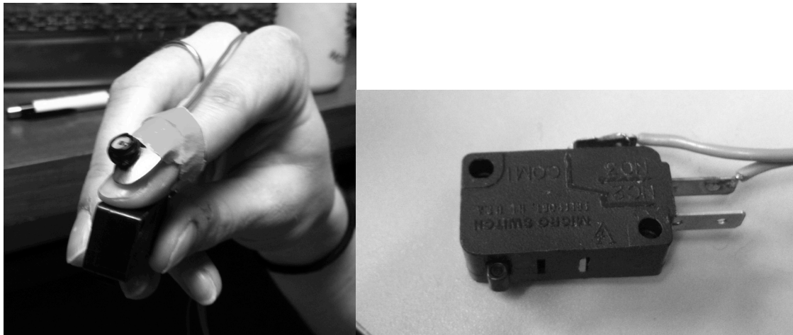
Figure 7 (left): Pinch grip with the infrared marker located above; Figure 8 (right): Mechanical trigger used as an input device for the E-Prime Software.
