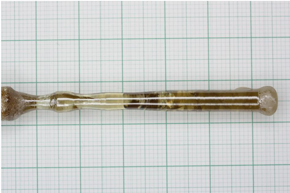
Figure 1.7: A single crystal of  $\text{Yb}_2\text{Ti}_2\text{O}_7$  we grew in an optical floating zone furnace at McMaster University. This sample was grown in 6 Atm of  $\text{O}_2$ . This crystal shows a color gradient possibly indicating  $\text{O}^{2-}$  defects.
