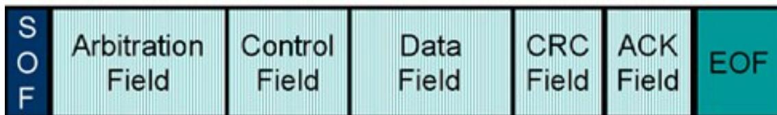
**Figure 2.5 CAN Bus Frame**
