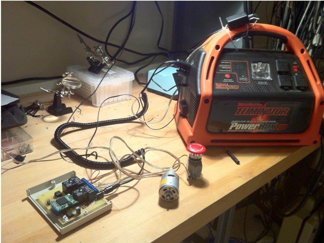
**Figure 5.4 Safety Circuit Bench Testing**
