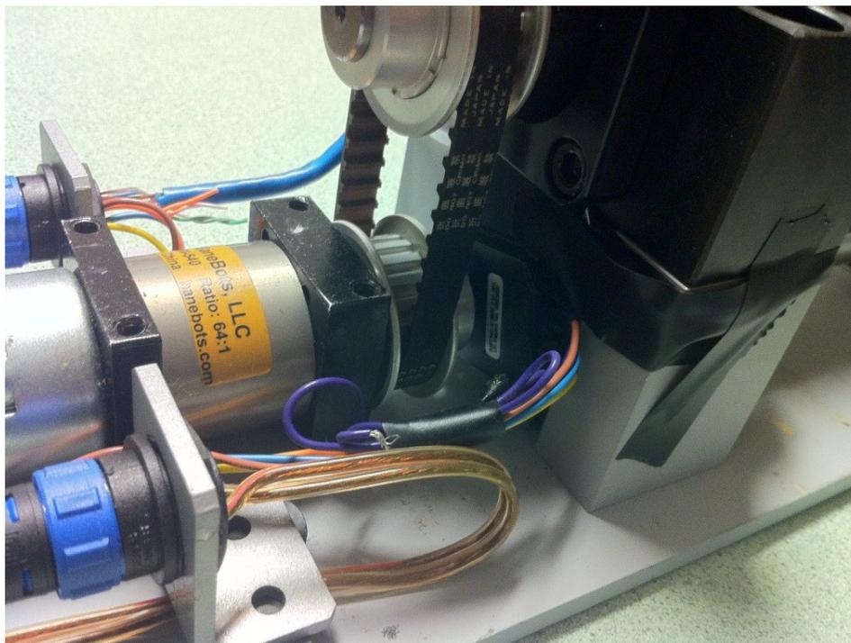
**Figure 5.6 Motor with Encoder**
