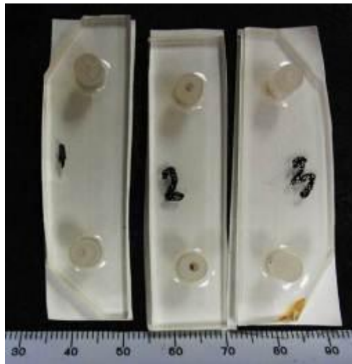
Figure 32: Microchannel test samples after treatment from 3H of SF 6 plasma
