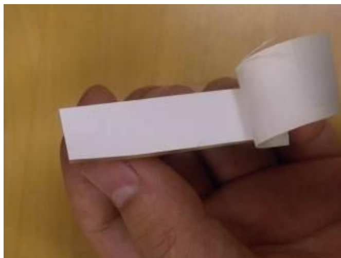
Figure 33: One year old sample treated with SF 6 plasma for three hours with backing peeled
