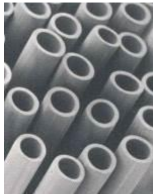
Figure 7: Commercial microporous polyethylene hollow fibers (www.mrc.co.jp)
