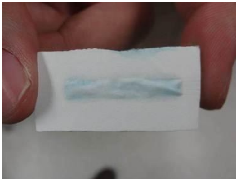
Figure 46: Permeation of water/ethanol in 3.3 mm large channel device during burst pressure test
