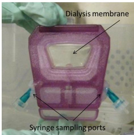
**Figure 0.6.** Depiction of a Slide-A-Lyzer cassette used for porewater extraction.
