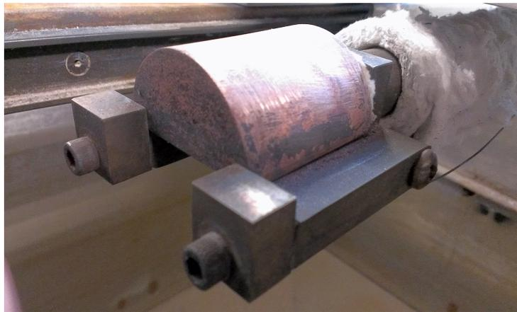
**Figure 6** – Specimen holder shown with a copper hemisphere clamped in place
