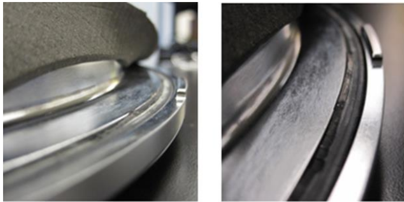
Figure 4. Foam ring applied over top of the rubber filled channel of the inner door plate of the PEA POD.
