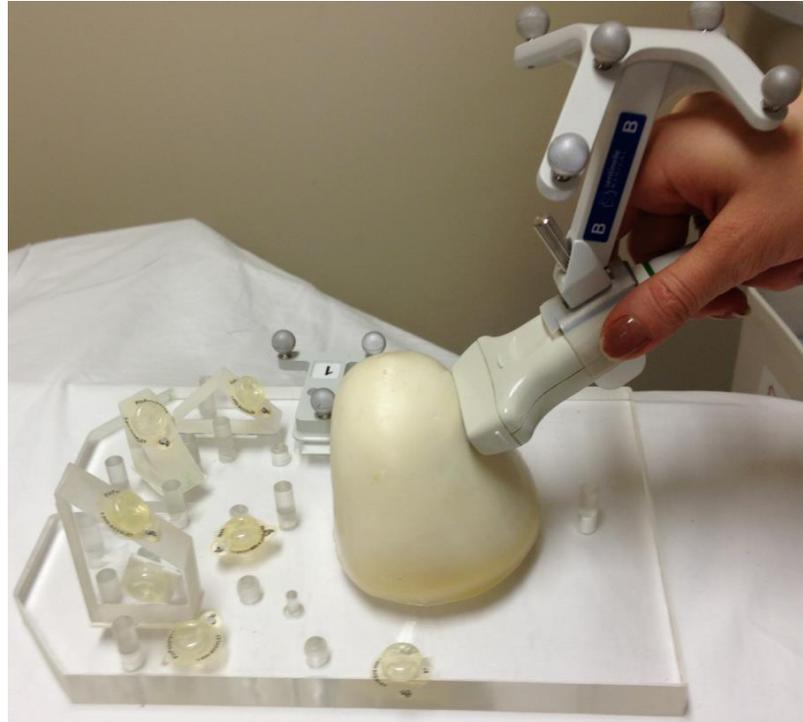
Figure 7.8: The breast phantom on the apparatus with fiducial markers and the US probe
