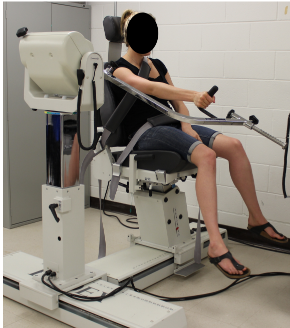
Figure 7: Example of the shoulder flexion-extension strength testing. The right shoulder angle was set and held at 60 degrees of elevation, in the frontal plane, with the elbow fully extended. The participant then applied maximal isometric force exertions while pulling up on the handle (flexion) and then pulling down on the handle (extension).
