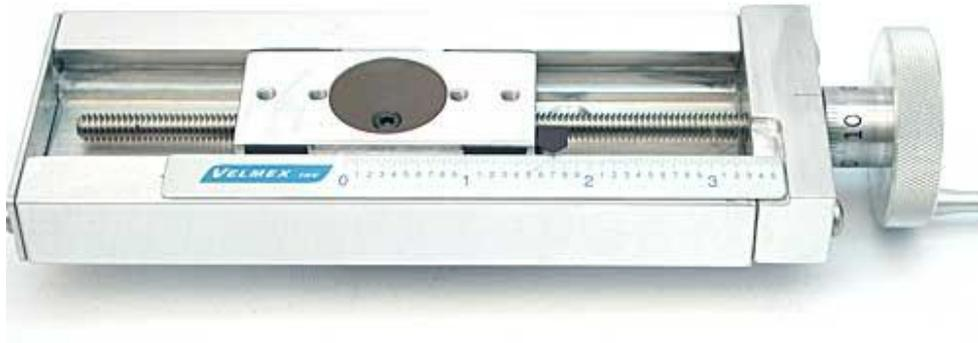
**Figure IV-2 Velmex™ 2.5 inch wide A25 series screw drive UniSlide Vice A2506P40-S2.5**
