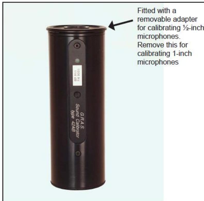
Figure IV-12 Sound Calibrator Type 42AB
