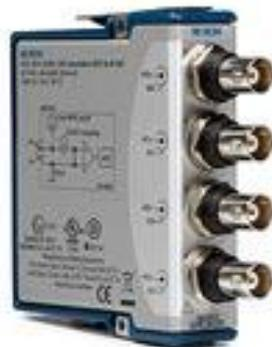
**Figure IV-14 National Instruments NI-9234 data acquisition**
