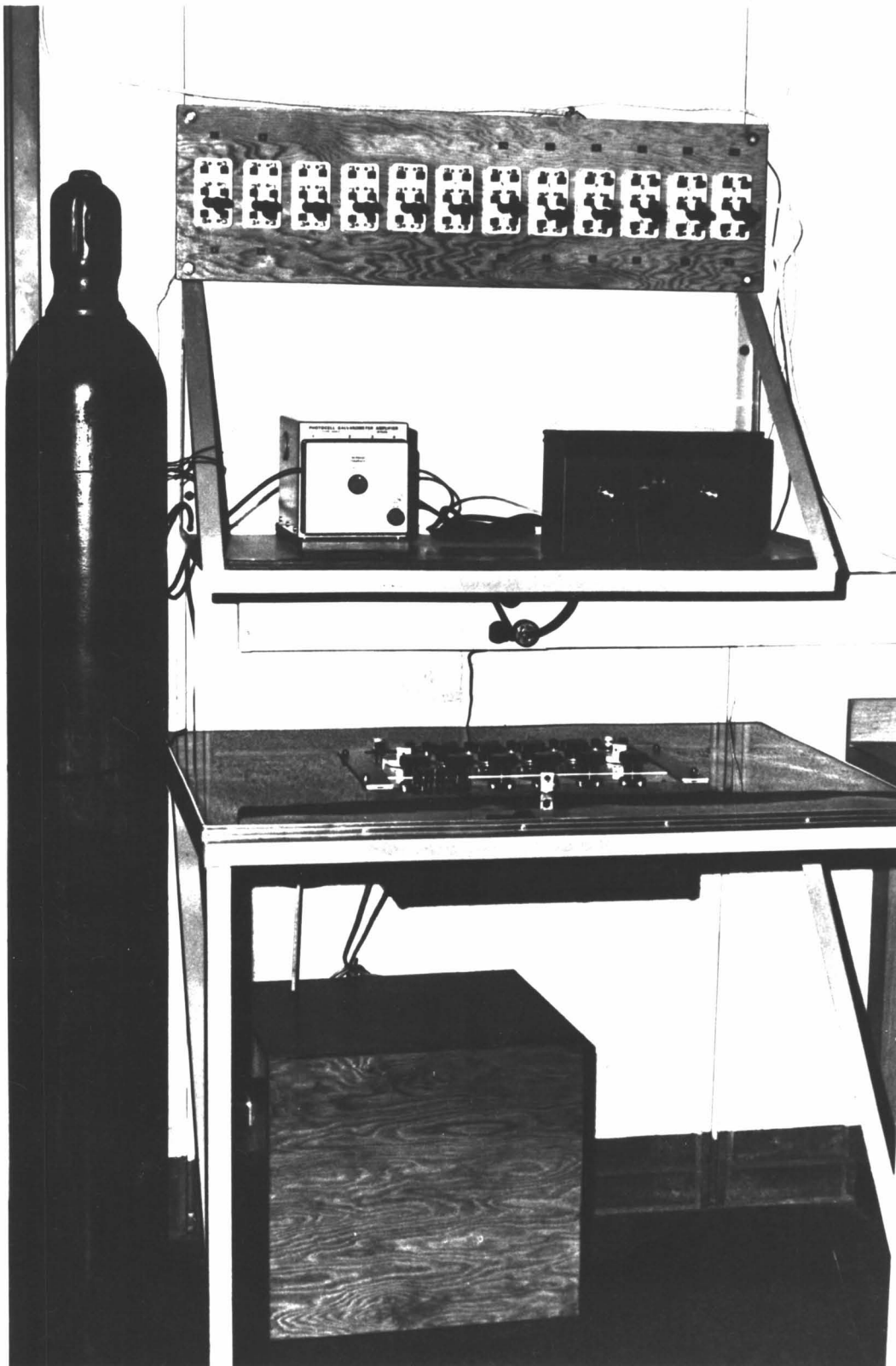
FIGURE 5. PHOTOCCELL GALVINOMETER POTENTIOMETER
