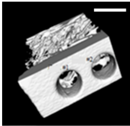
Figure 38: Micro-CT image for two holes were ablated by concentric circle scanning, hole#1 has 20 layers and hole#2 has 10 layers, the successive layers were separated by 200 \mu\text{m} distance in both holes, (scale bar = 1 mm)
