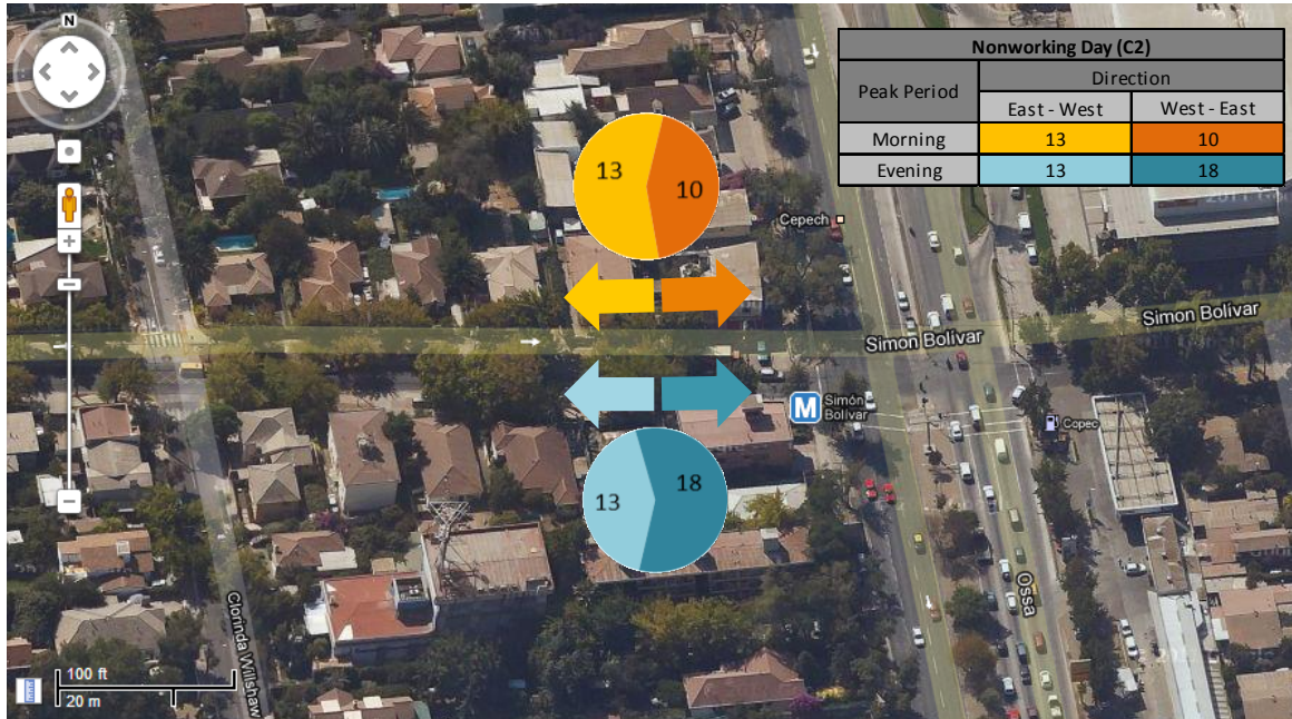
Figure 22. Flow Diagram for peak times. Non-working day, Simon Bolivar cycle lane (C2)
