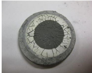
(S15) 67%: program 1+ sintering (1h), 0.5h wet H_2 (900°C- 1100°C), 1h dry H_2 (1300°C)
