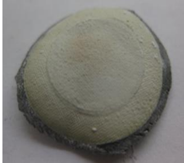
(S76) Group 1:56%: burning out + sintering (6h), 3h wet H_2 and 3h dry H_2 (1100°C)
