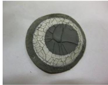
(S3) 67%: program 1+ sintering (4h), 1.5h wet H_2 and 2.5h dry H_2 (1300°C)
