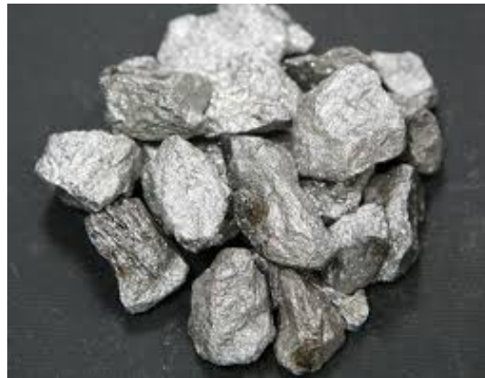
Figure 8 – A sample of standard grade ferroniobium produced by CBMM
