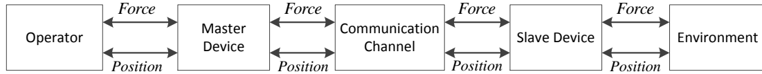
Figure 1.2: Block diagram of a symmetric SMSS teleoperation system. The master and slave blocks contain the respective device and its controller.
