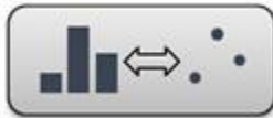
Figure 10 Button that allows users to switch between bar graphs (confidence values off) and bubble plots (confidence values on)
