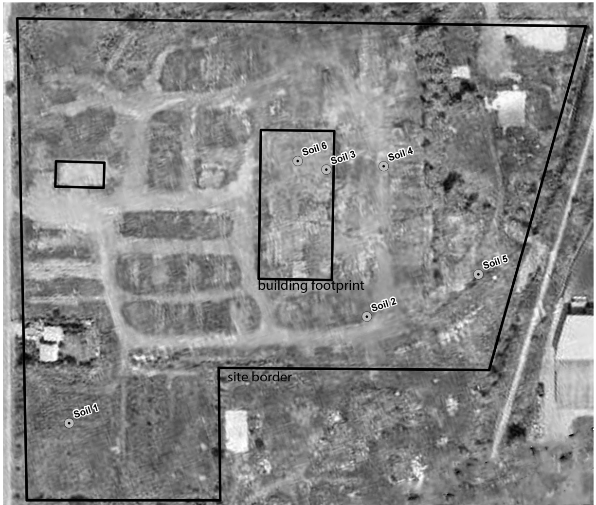
Figure 3.S1 Sampling locations for soils 1 to 6 from industrial processing site. Former building footprints are outlined in black.
