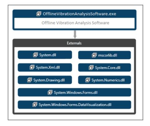
Figure 4.3: Offline Vibration Analysis Software Dependencies
