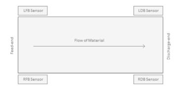
Figure 2.1: Measurement Locations on a Two Bearing Machine
