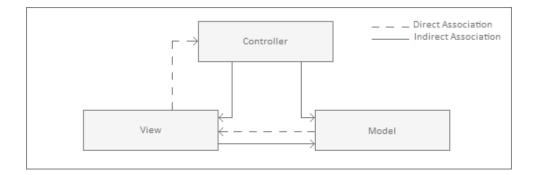
Figure 4.4: Model View Controller Architecture
