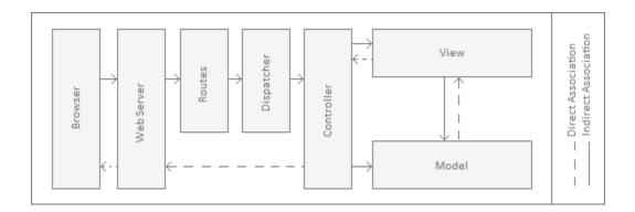
Figure 5.1: ASP.NET MVC Framework
