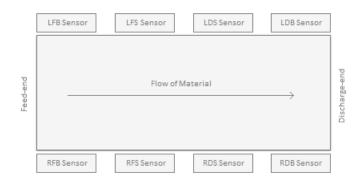
Figure 2.2: Measurement Locations on a Four Bearing Machine
