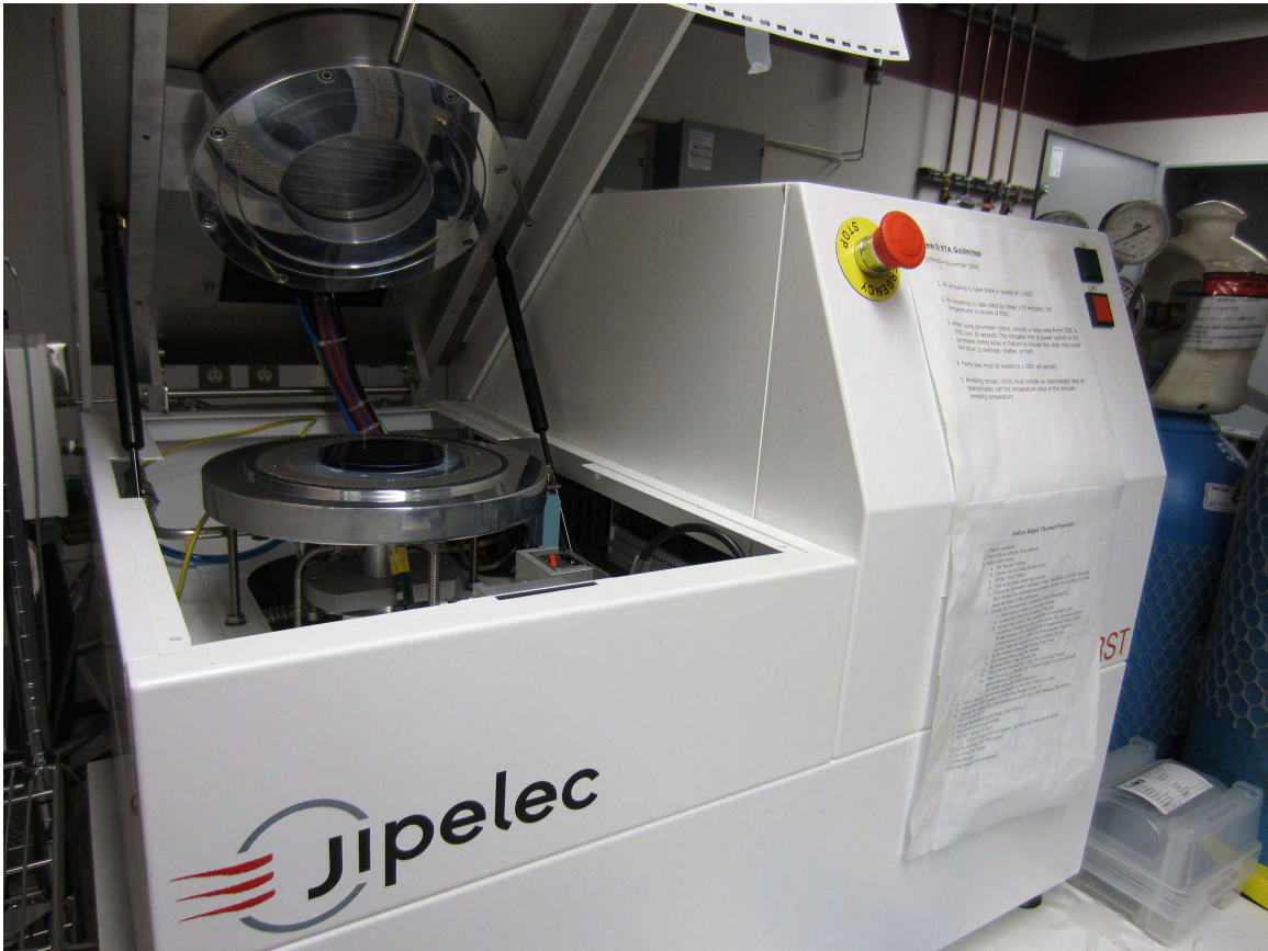
Figure 3.2: Photograph of the Qualiflow Jipelec Jetfirst 100 rapid thermal processor used in the isothermal annealing studies of silicon-rich silicon nitride films.
