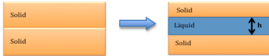
Figure 2.3: A premelted grain boundary, where h is the film width
