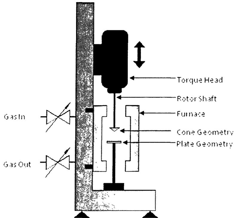
**Figure 5:** Schematic of the rotational rheometer (AR2000) outfitted with a cone and plate measurement geometry
