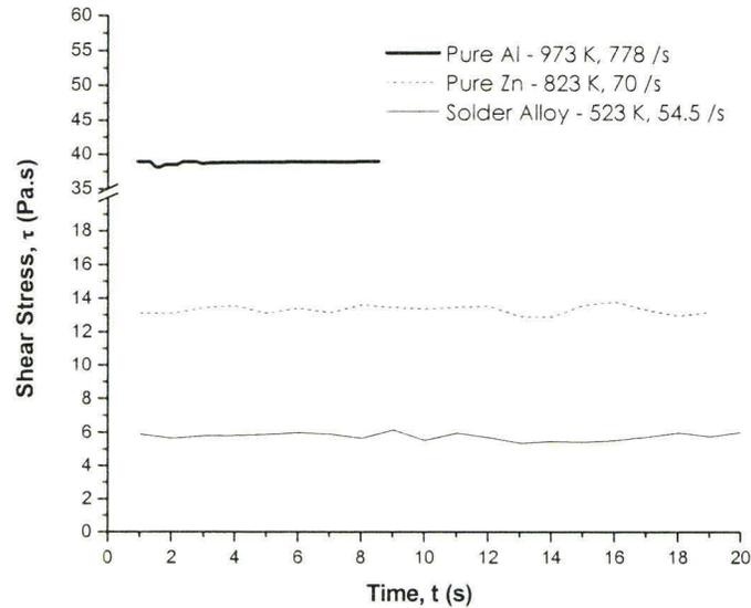
**Figure 8:** Time dependency Curve (shear stress versus time) for liquid metal systems at specific melt temperature and shear rate.
