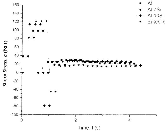
**Figure 8:** Time dependency curve (Shear stress versus time) for liquid Al-Si alloy system at specific melt temperature and shear rate
