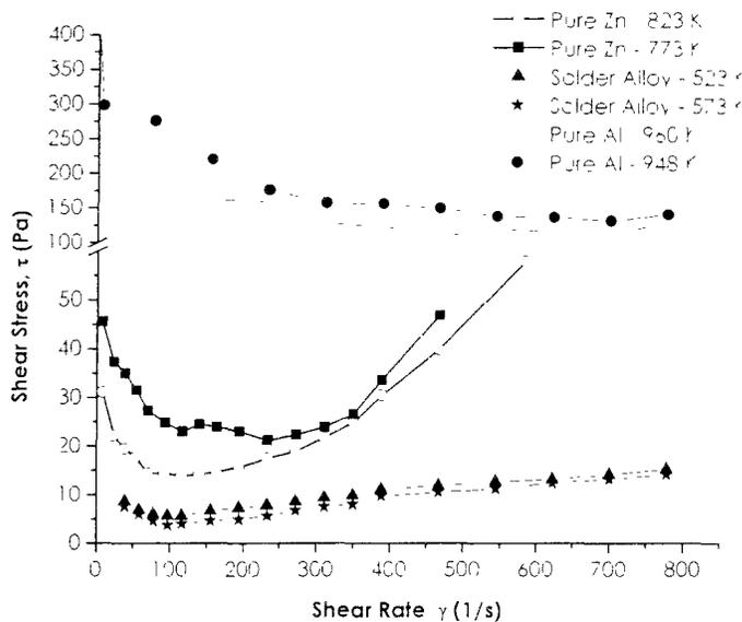
**Figure 9:** Flow Curves (shear stress versus shear rate) for liquid metal systems at various melt temperatures.
