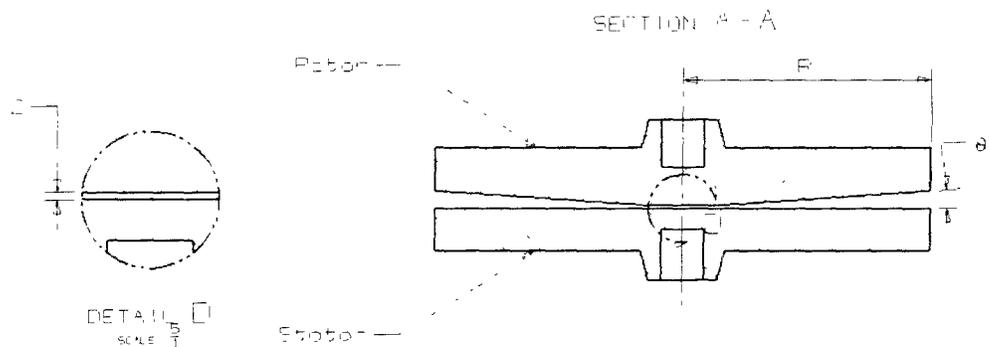
**Figure 2:** Cross-section of Cone and Plate measurement geometry. The liquid is contained between the rotor and stator
