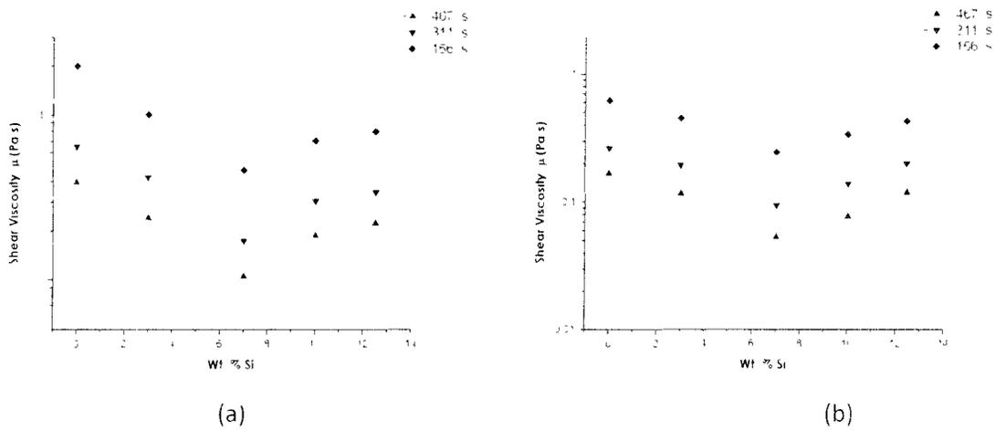
**Figure 11:** Viscosity as a function of Si content for three different shear rates (a) 5K melt superheat temperature and (b) 973K
