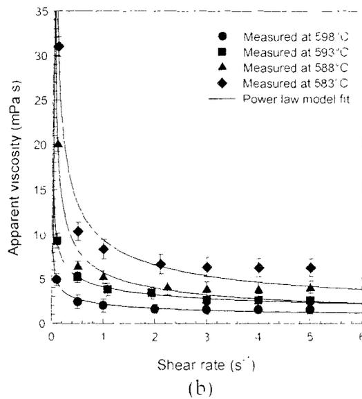
Figure 9: Results from rotational rheometer experiments with cone and plate for molten Al-12.5 wt% Si alloys. (a) Flow curves at four melt superheats. (b) Apparent viscosity data as a function of shear rate and melt superheats.
