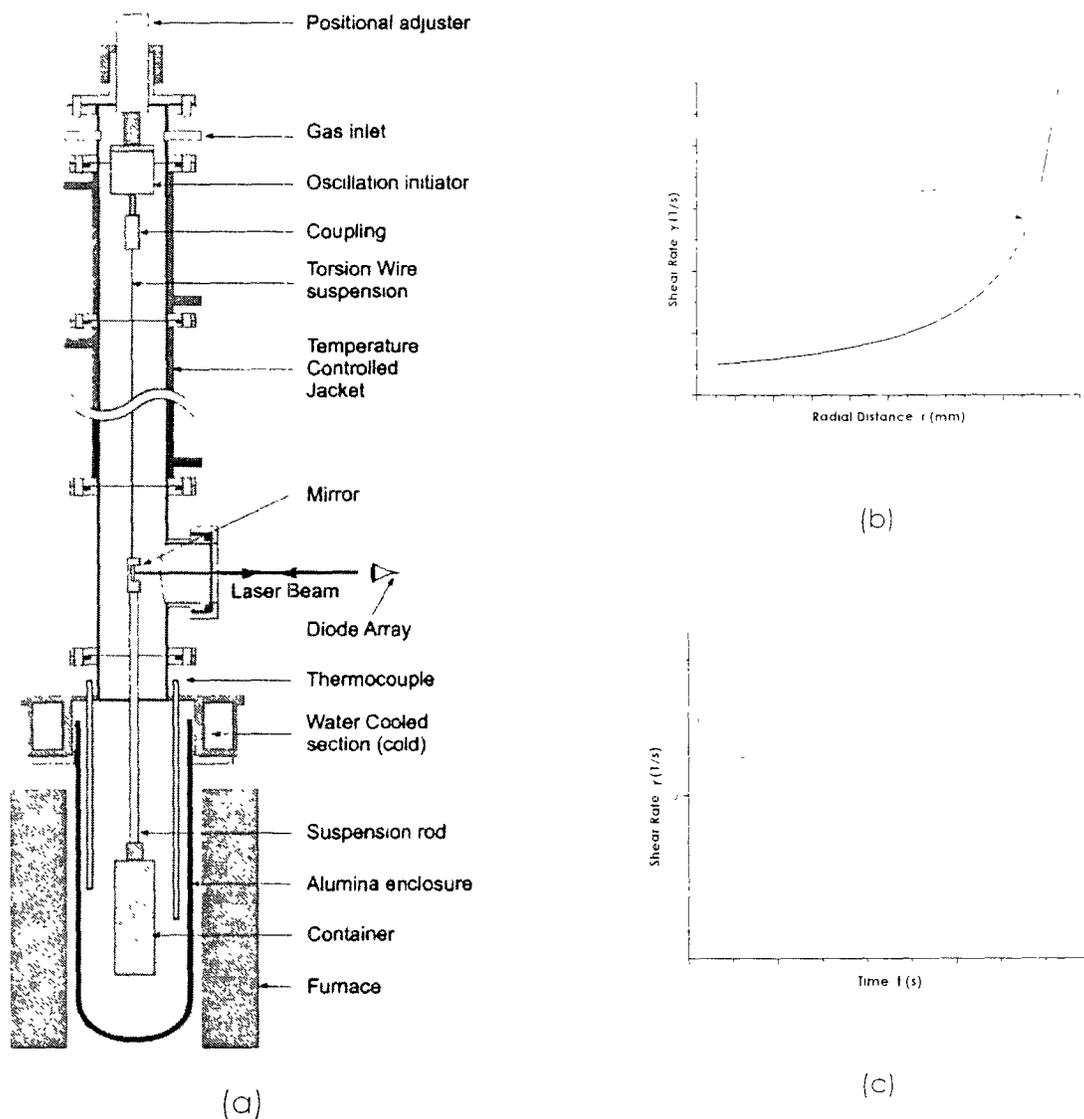
**Figure 1:** Schematic of a typical (a) Oscillating Vessel Viscometer (OVV) (b) the spatial variation of shear rate, and (c) the temporal variation in shear rate
