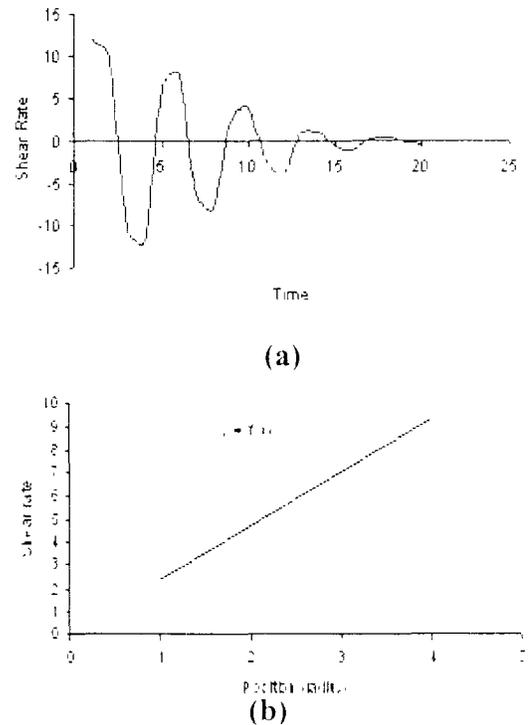
**Figure 3: Schematic graphical representation of the variation of shear rate in an oscillation vessel viscometer. (a) Temporal variation and (b) Spatial variation.**
