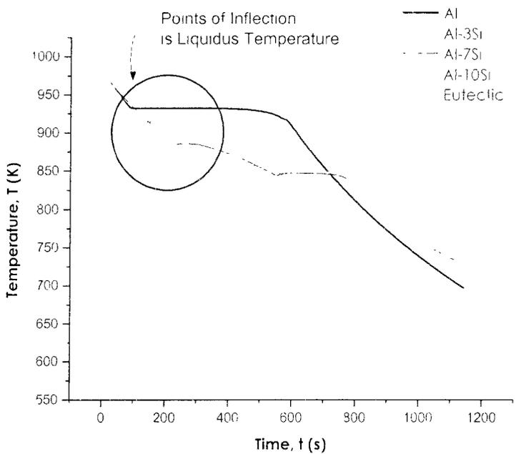
Figure 6: Thermal data during solidification of the alloys presented in Table I.
