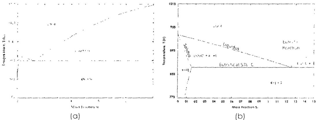
**Figure 2:** Al-Si binary alloy phase diagram. (a) the complete phase diagram for 0 to 1 mass fraction Si and (b) magnified region showing the hypoeutectic alloy between 0 and 0.125 mass fraction Si.
