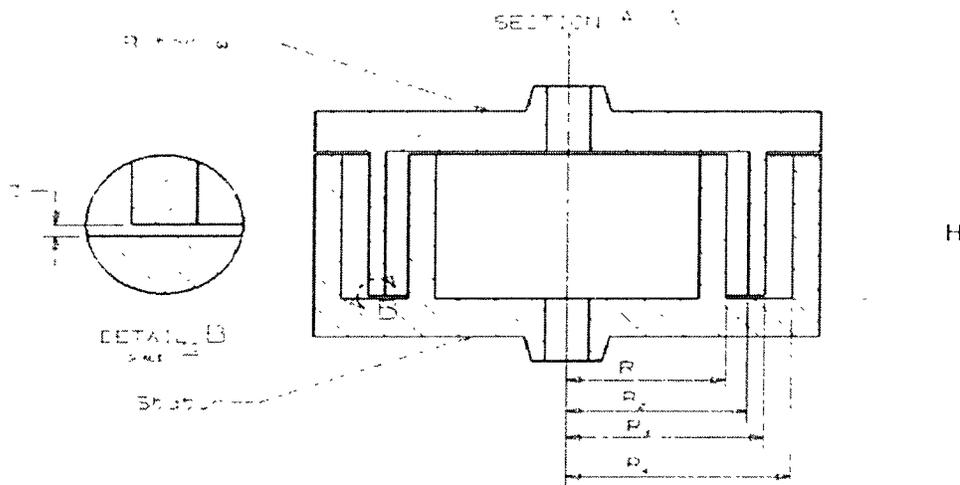
**Figure 2:** Cross-section of Double Concentric Cylinder (DCC) measurement geometry used in the present experiment study.  $R_1 = 14.5$  mm,  $R_2 = 16.5$  mm,  $R_3 = 18$  mm,  $R_4 = 20.5$  mm,  $H = 15$  mm and  $z = 0.30$  mm.
