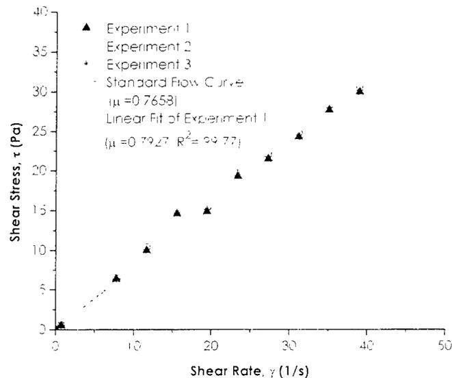
**Figure 7:** Flow Curve (shear stress versus shear rate) for Cannon S2000 standard liquid showing repeatability and accuracy of the rheometer.
