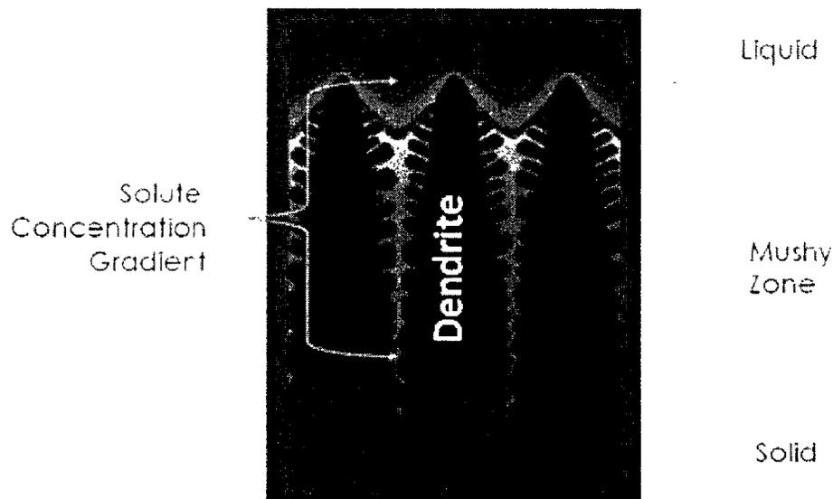
**Figure 3:** Typical schematic of the microstructure developed during solidification of Al-Si hypoeutectic binary alloy.
