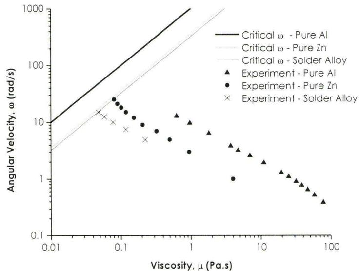
**Figure 6:** Representation of Taylor Vortex Criteria for three liquid metal systems. The solid lines is the plot of the critical angular velocity as a function of shear rate above which vortices will form in the respective sheared liquids during rotational rheometry with the DCC geometry shown in Figure 4. The data points are the actual experiments carried out in this study showing that Taylor vortices may not form in the sheared liquids during the experiments.
