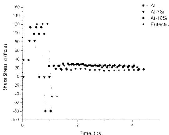
**Figure 4:** Time dependency curves (Shear stress versus time) for liquid Al-Si alloy modified system at specific melt temperature and shear rate
