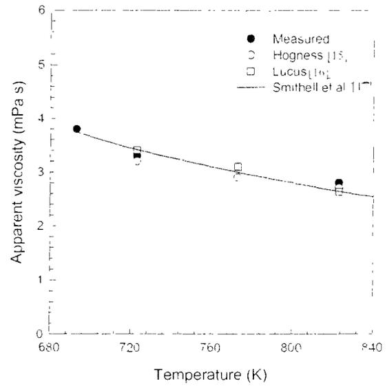
Figure 8: Results from rotational rheometer experiments with cone and plate for 99.99 % purity molten Zn. (a) Flow curves and (b) Apparent viscosity as a function of temperature [16,17,18].
