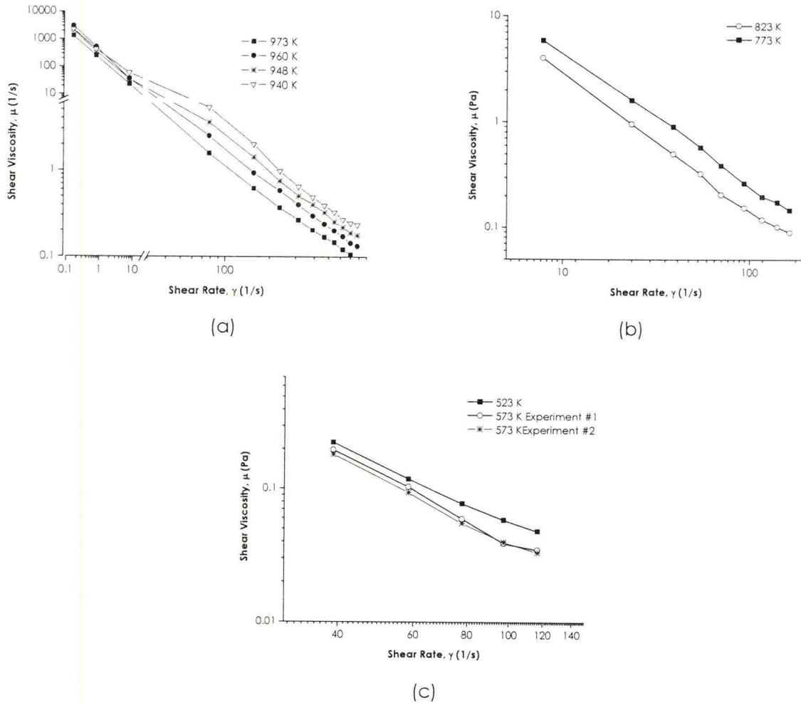
**Figure 10:** Viscosity curves of liquid metal systems as a function of shear rate at various melt temperatures. (a) pure Al, (b) pure Zn and (c) Sn<sub>95.8</sub>Ag<sub>3.28</sub>Cu<sub>0.92</sub> solder alloy.
