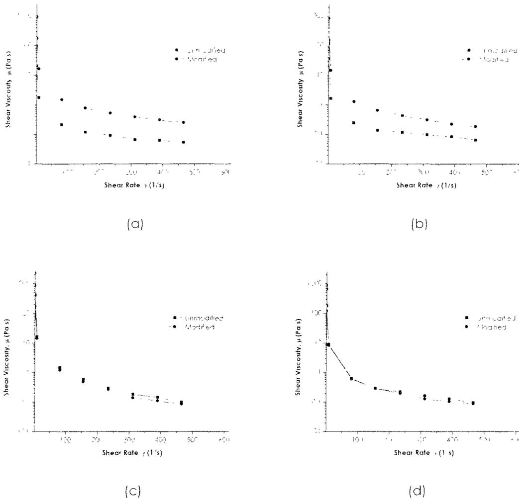
**Figure8:** Comparison of viscosity versus shear rate for modified and unmodified Eutectic (a) 858K, (b) 878K, (c) 948K, and (d) 973K
