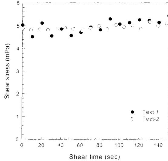
**Figure 7: Relationship between shear stress and shear time for the Al-12.5wt%Si alloy tested at  $\dot{\gamma} = 0.5 \text{ s}^{-1}$  and  $598^\circ\text{C}$ .**
