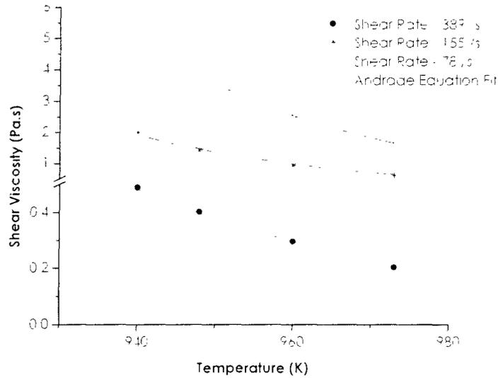
**Figure 11:** Viscosity at various shear rates as a function of melt temperature for liquid pure Al. Also shown is the curve fit to the data points for each shear rate with Andrade's equation shown in Equation (16)
