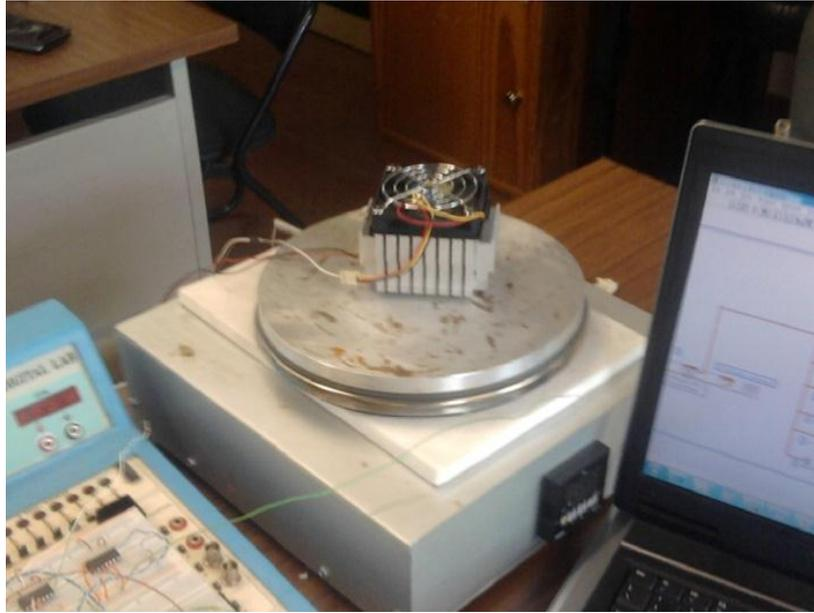
**Figure 2.9 Experimental Facility used to characterize the performance of thermoelectric generators Carmo[29]**
