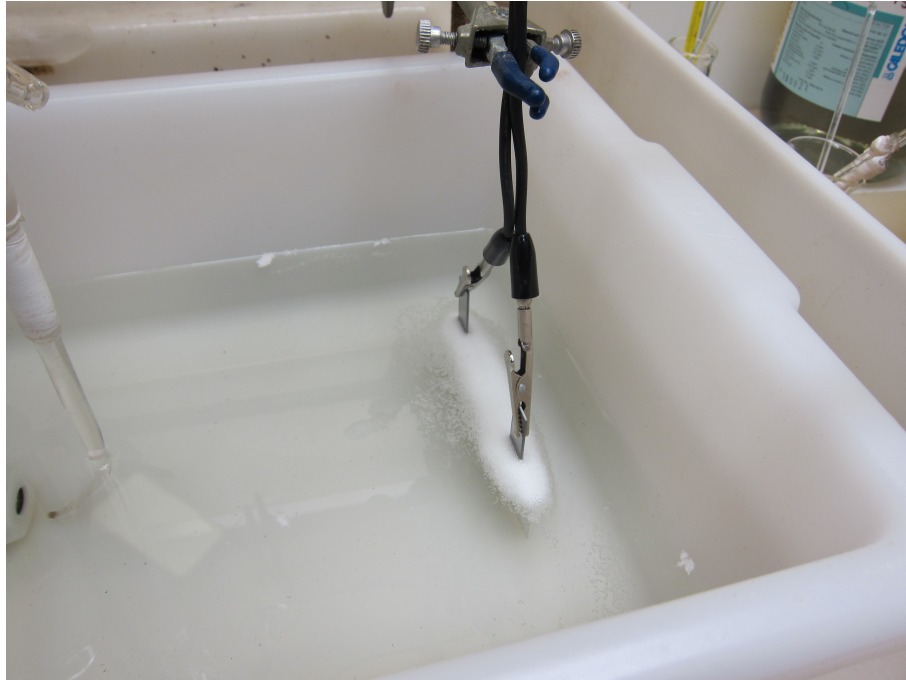
Figure 14: Galvanic couple surface area experiment
