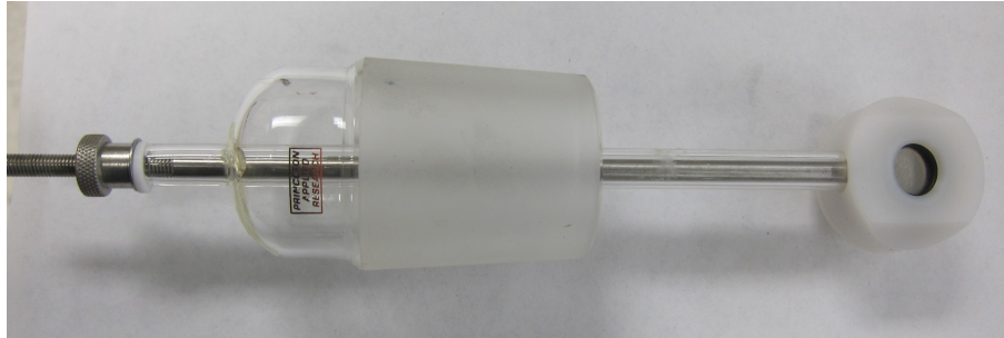
Figure 10: Princeton Research K105 Flat Specimen holder® with a Kalrez® washer
