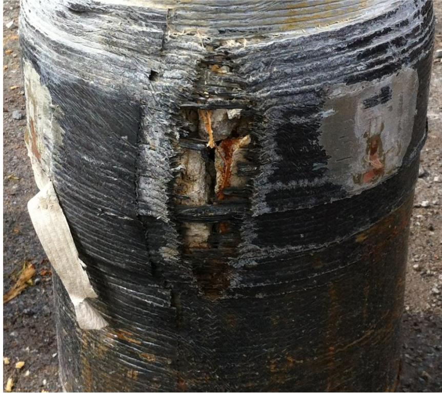
Figure 2.24: C4-2 CFRP Rupture Location
