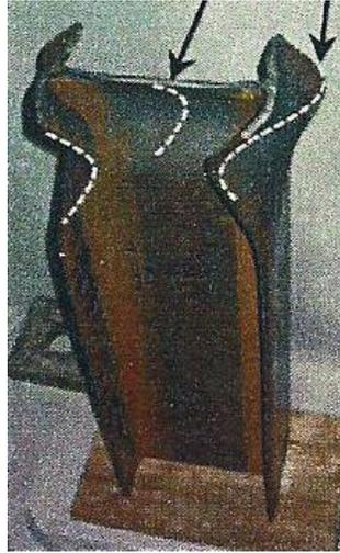
Figure 2.20: C1 – Steel Section Failed Specimen (From Karimi et al. (2010))
