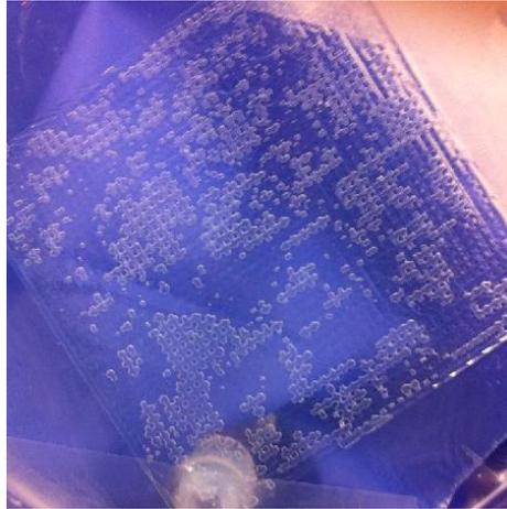
**Figure 27.** Microchannel grid showing regions blocked by air bubbles when PBS was circulated.
