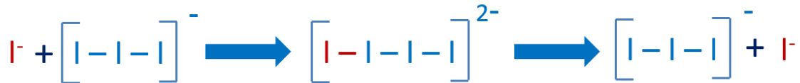
Figure 1.12: The Grotthuss-like mechanism in a highly concentrated (ionic liquid) electrolyte based on I^-/I_3^- redox couple
