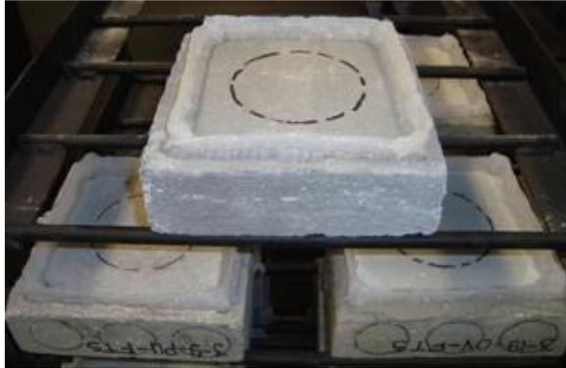
**Figure 3.11 Freeze-thaw with salt solution specimens**
