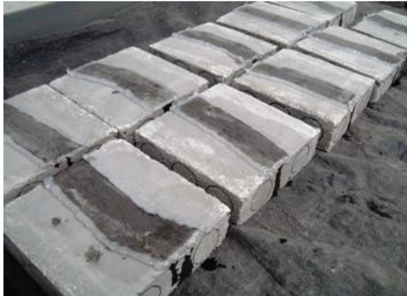
**Figure 3.7 Epoxy poured into silicone dikes**
