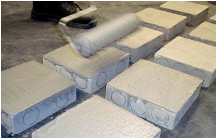
**Figure 3.9 Application of the first layer of SikaTop Seal 107**
