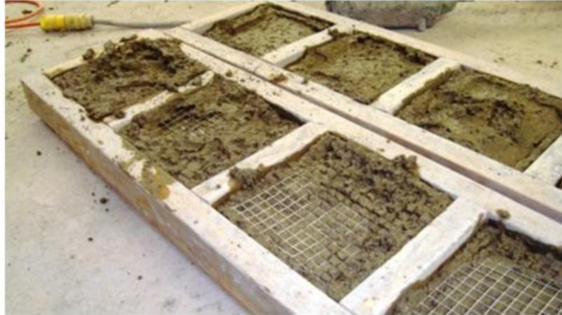
**Figure 3.4 Steel mesh placement in concrete specimens**
