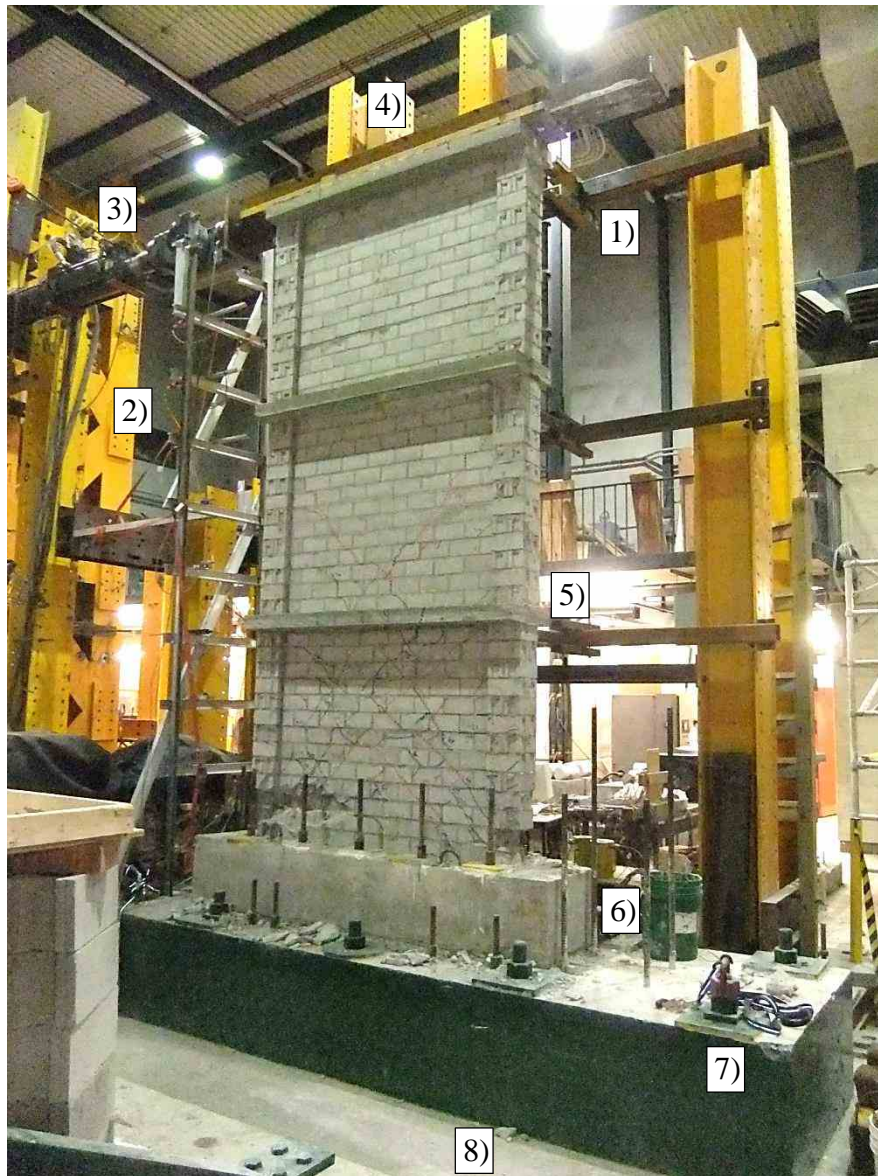
Figure 2.6 – Photo of Test Set-Up with Wall 9 at End of Test: 1) Top of Wall Out-of-Plane Support, 2) Reaction Frame, 3) \pm 500 kN & 500 mm Stroke Hydraulic Actuator, 4) Rigid Steel Loading Beam fixed to Top of Wall, 5) 4 \times Inter-Storey Out-of-Plane Supports, 6) RC Wall Footing, 7) Reusable RC Base, 8) Strong Floor
