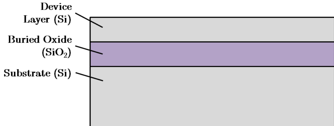
Figure 1.1: Illustrated cross-section of a silicon-on-insulator (SOI) wafer. The thickness of the device layer typically ranges from hundreds of nanometres to a few micrometres. The thickness of the buried oxide layer is typically one to two micrometres.
