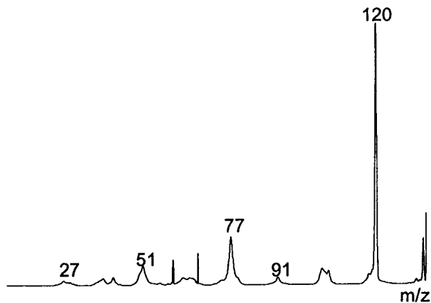
Figure 7-6: CID mass spectrum (2ffr, 8 keV, collision gas O 2 ) of ionized N-ethyl-N-methylaniline, m/z 135.
