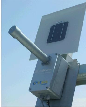
Figure 4.3 - A tracking accuracy sensor mounted on one of Inspira’s CPV lab tracker [50].
