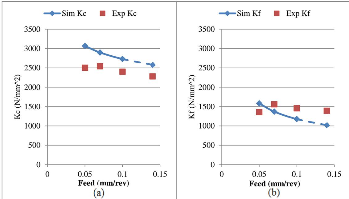
Figure 5-19: Simulation and Experimental results (a) cutting coefficient  $K_c$  (b) cutting coefficient  $K_f$ . cutting speed  $v=100$  m/min
