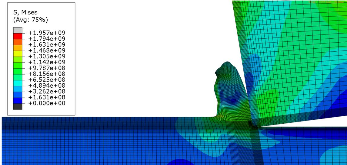
Figure 3-9: Chip formation  $f=0.05$  mm/rev,  $v=100$  m/min and  $\rho_e=60$   $\mu\text{m}$
