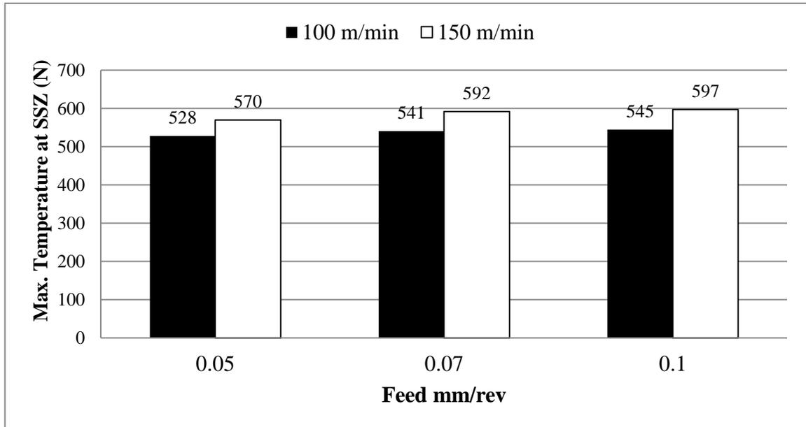
Figure 5-14: Maximum temperature at the SSZ at  $v= 100$  m/min and  $v= 150$  m/min at different feed rates (simulation results only)
