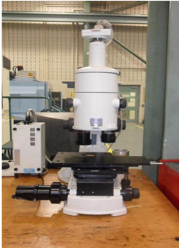
Figure 4-8: Nikon AZ100 microscope for measuring the tool rake angle
