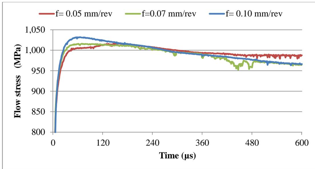
Figure 5-15: flow stress at feed rates  $f = 0.05$ ,  $f = 0.07$  and  $f = 0.10$  mm/rev.
