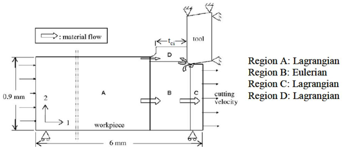
Figure 2-8: Boundary conditions, partitioning scheme and material flow when employing ALE [33]
