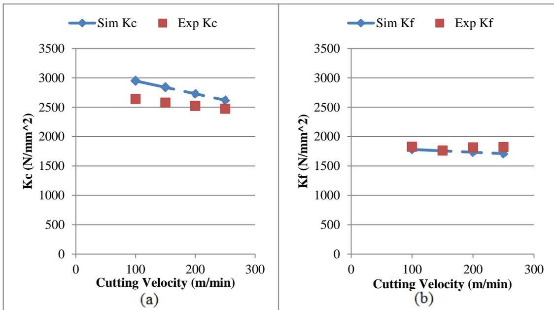
Figure 5-8: Simulation and Experimental results (a) cutting coefficient  $K_c$  (b) cutting coefficient  $K_f$ . Feed rate  $f= 0.07$  mm/rev
