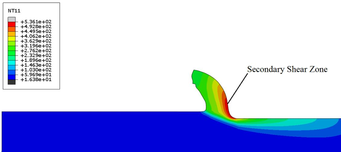
Figure 5-2: Thermal distribution for workpiece at  $f= 0.05$  mm/rev and  $v= 100$  m/min
