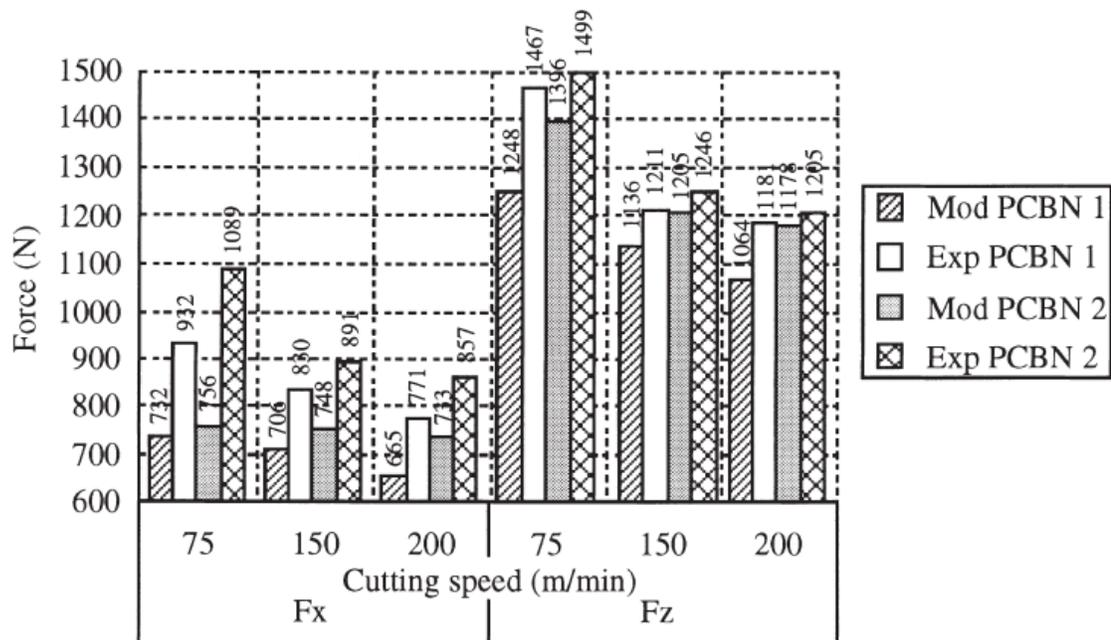
Figure 2-13: Comparison between model and experimental data on the effect of cutting speed on the feed force  $F_f$  and tangential force  $F_c$  (referred to as  $F_x$  and  $F_z$ ) [41]
