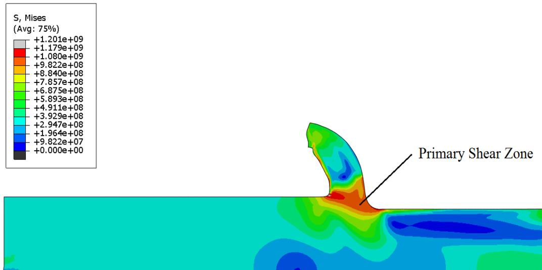
Figure 5-1: Stress distribution for workpiece at  $f = 0.05 \text{ mm/rev}$  and  $v = 100 \text{ m/min}$
