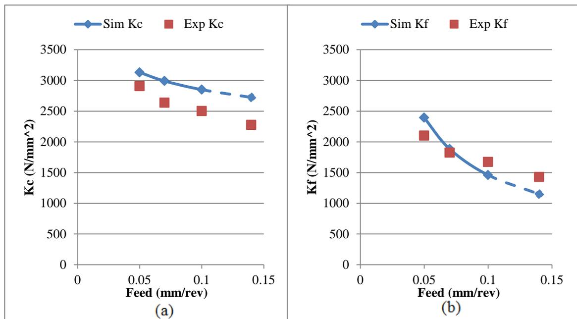
Figure 5-5: Simulation and Experimental results (a) cutting coefficient  $K_c$  (b) cutting coefficient  $K_f$ . Cutting speed  $v=100$  m/min
