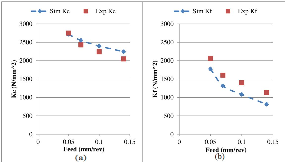
Figure 5-25: Simulation and Experimental results (a) cutting coefficient  $K_c$  (b) cutting coefficient  $K_f$ . cutting speed  $v=250$  m/min
