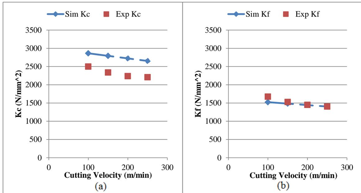
Figure 5-9: Simulation and Experimental results (a) cutting coefficient  $K_c$  (b) cutting coefficient  $K_f$ . Feed rate  $f=0.10$  mm/rev
