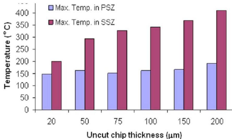
Figure 2-16: Variation of maximum temperature in the primary and secondary shear zones at 200 m/min cutting speed, PSZ: primary shear zone, SSZ: secondary shear zone [45]
