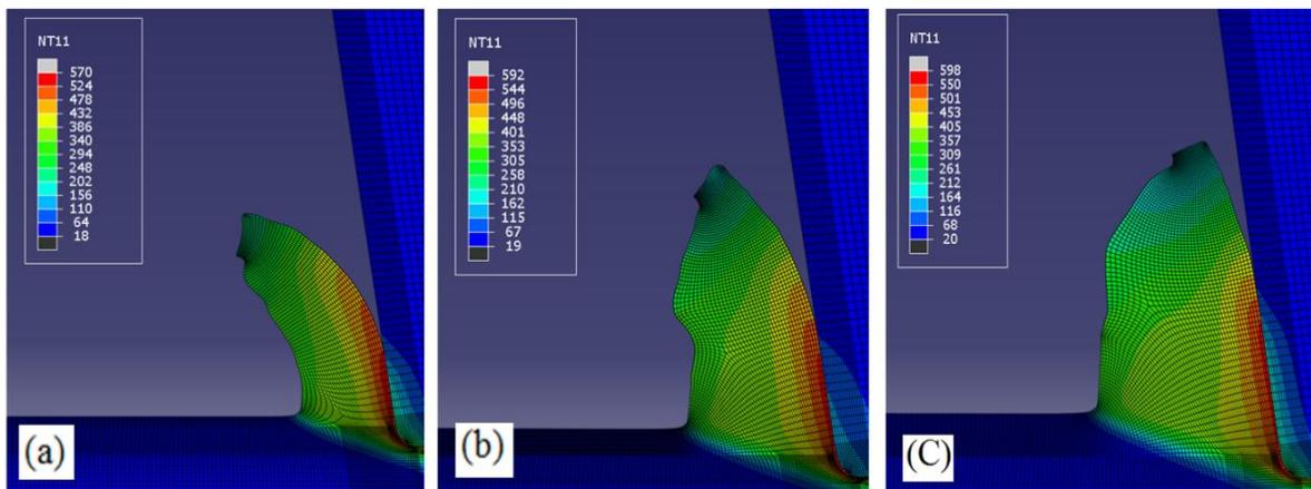
Figure 5-13: Temperature of SSZ at  $v=150$  m/min (a)  $f=0.05$  mm/rev (b)  $f=0.07$  mm/rev (c) rate  $f=0.10$  mm/rev
