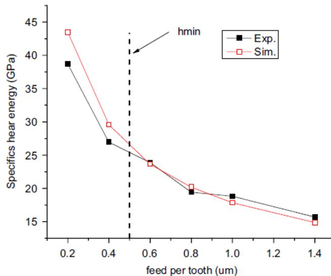
Figure 2-12: Size effect in specific shear energy at different feed rates [5]
