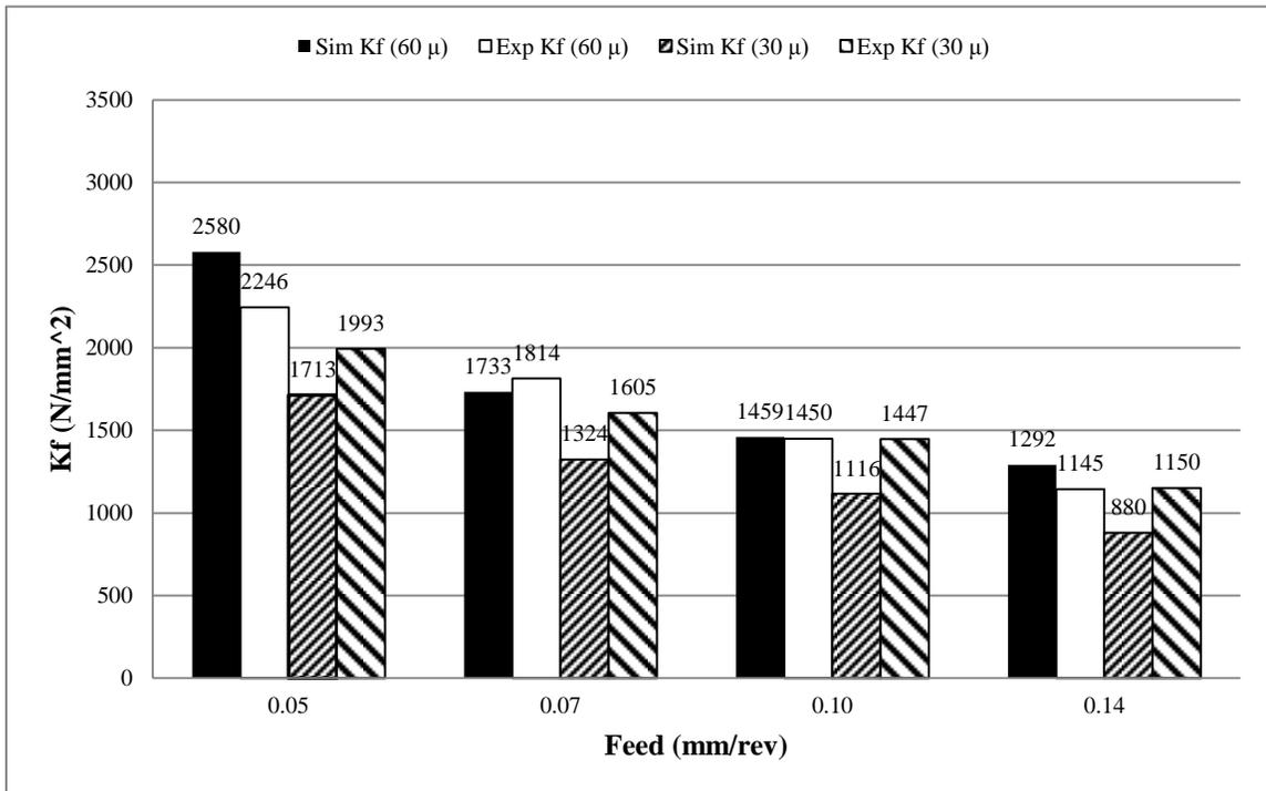
Figure 5-34: Effect of cutting edge radius on  $K_f$  at  $v=200$  m/min
