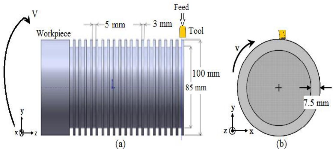
Figure 4-3: Workpiece Geometry
