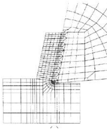
Figure 2-6: Example of initial geometry using Eulerian formulation [24]
