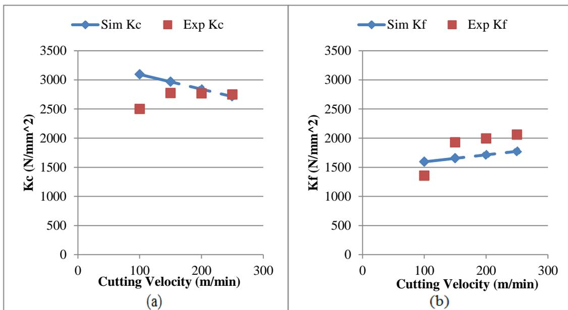
Figure 5-21: Simulation and Experimental results (a) cutting coefficient  $K_c$  (b) cutting coefficient  $K_f$ . Feed rate  $f = 0.05$  mm/rev
