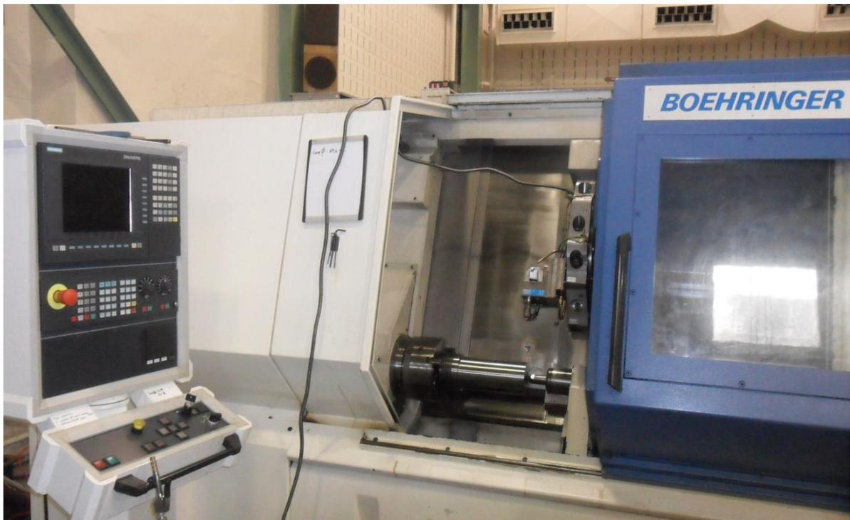
Figure 4-1: Boehringer VDF 180CM (CNC) lathe
