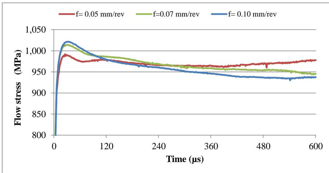
Figure 5-16: flow stress at feed rates  $f = 0.05$ ,  $f = 0.07$  and  $f = 0.10$  mm/rev.
