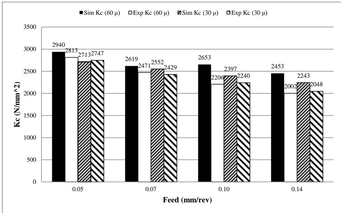
Figure 5-35: Effect of cutting edge radius on  $K_c$  at  $v = 250$  m/min
