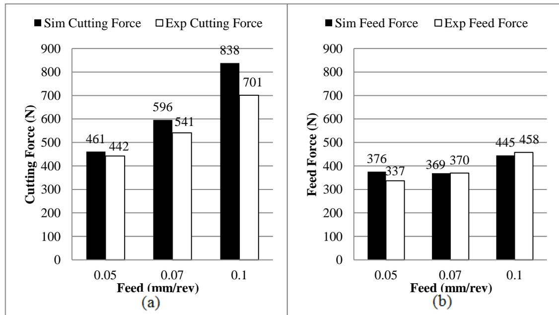
Figure 5-4: Simulation and Experimental results (a) Cutting force  $F_c$  (b) feed force  $F_f$ .
