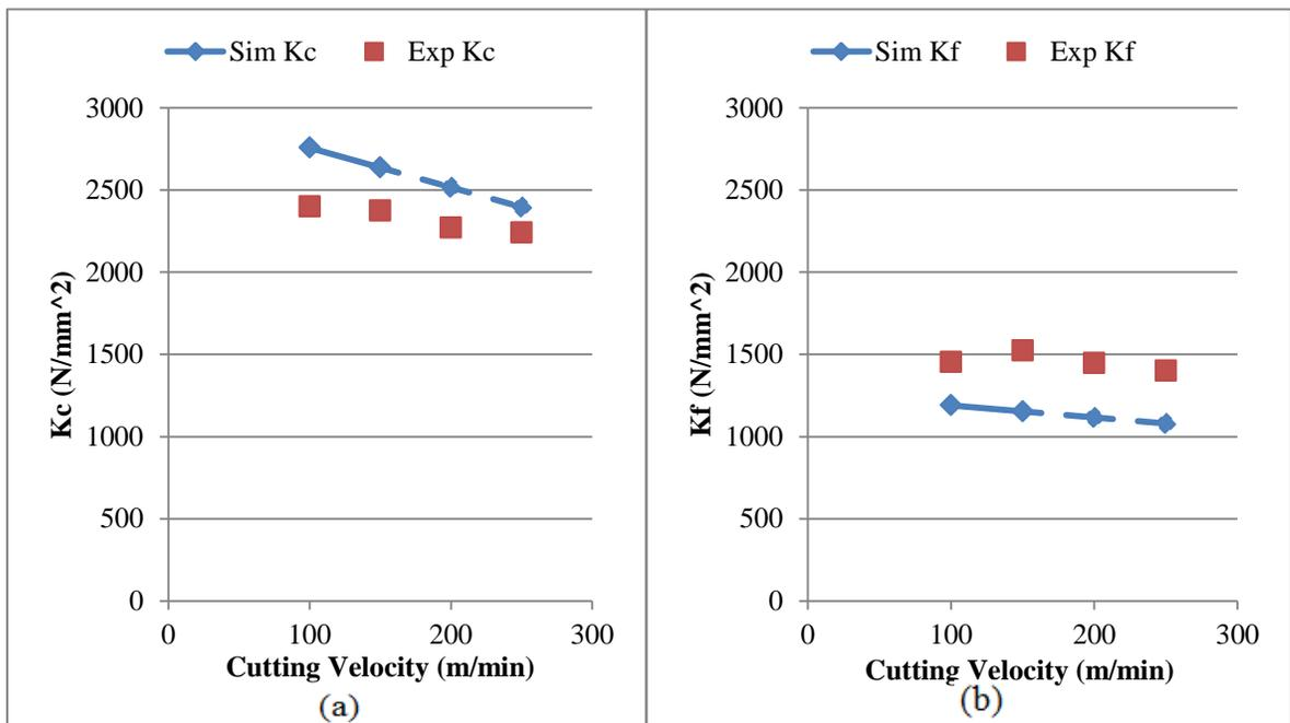
Figure 5-23: Simulation and Experimental results (a) cutting coefficient  $K_c$  (b) cutting coefficient  $K_f$ . Feed rate  $f = 0.10$  mm/rev
