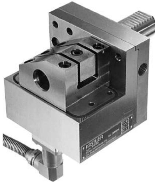
Figure 4-10: Kistler type tool-post piezoelectric dynamometer
