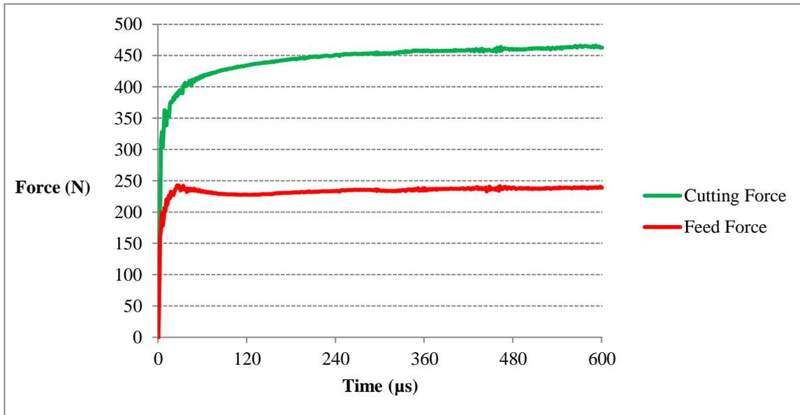
Figure 3-10: Cutting and Feed forces  $F_c$  and  $F_f$   $f=0.05$  mm/rev,  $v=100$  m/min and  $\rho_e=60$   $\mu\text{m}$
