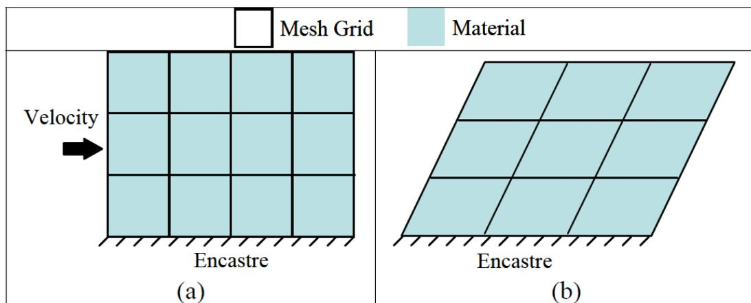
Figure 2-3: Initial position of mesh grids and material. (b) Both material and element mesh grid deformation after the velocity is applied [9]
