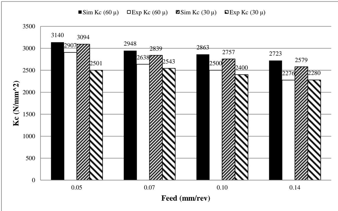
Figure 5-29: Effect of cutting edge radius on  $K_f$  at  $v=100$  m/min
