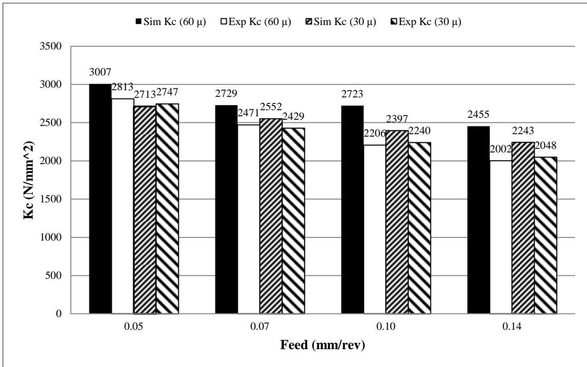
Figure 5-33: Effect of cutting edge radius on  $K_c$  at  $v=200$  m/min
