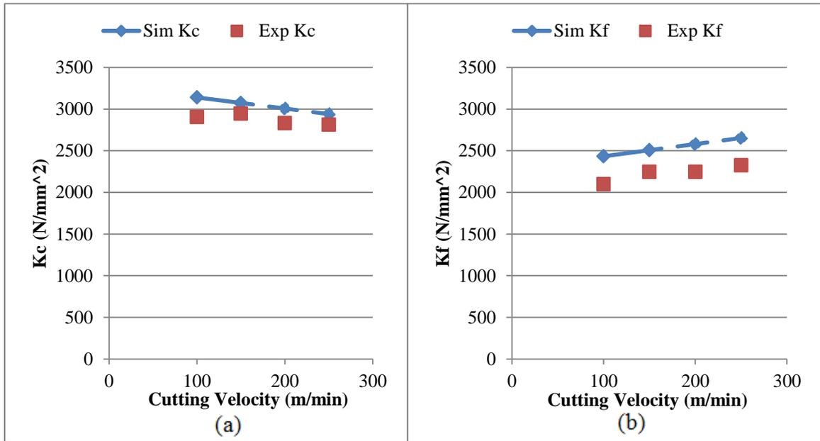
Figure 5-7: Simulation and Experimental results (a) cutting coefficient  $K_c$  (b) cutting coefficient  $K_f$ . Feed rate  $f= 0.05$  mm/rev
