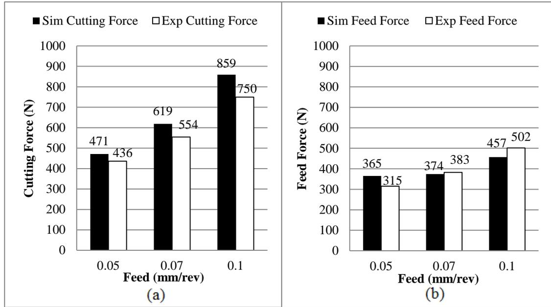
Figure 5-3: Simulation and Experimental results (a) Cutting force  $F_c$  (b) feed force  $F_f$ . Cutting speed  $v=100$  m/min
