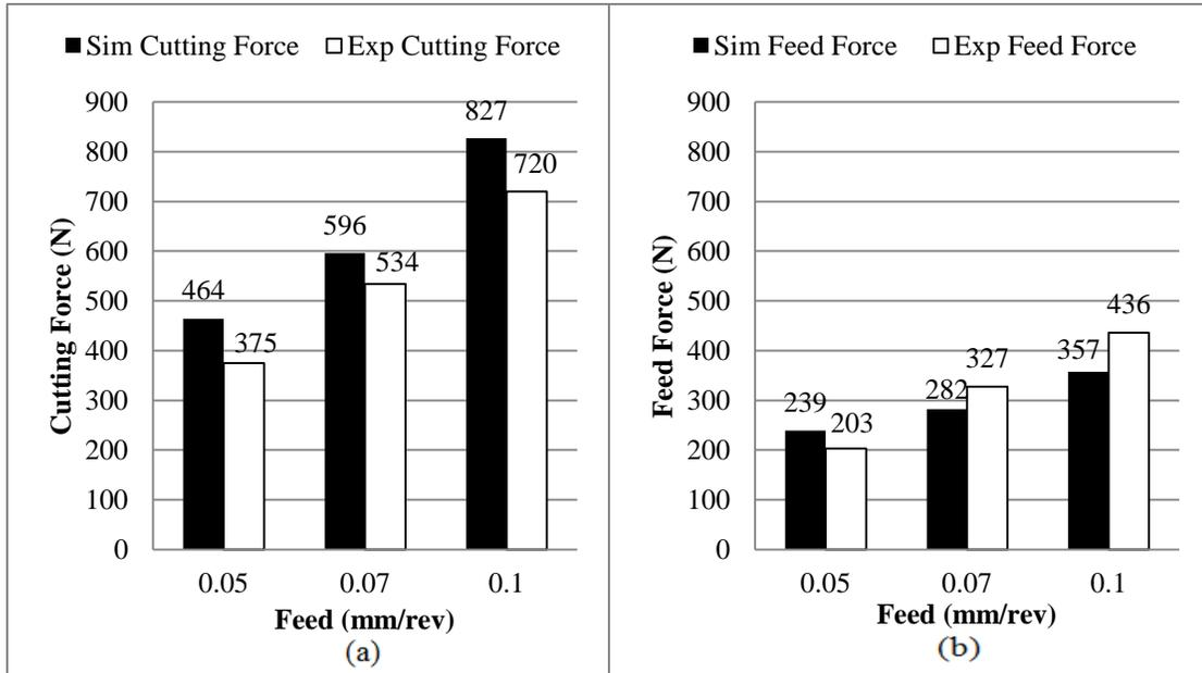
Figure 5-17: Simulation and Experimental results (a) Cutting force  $F_c$  (b) feed force  $F_f$ . Cutting speed  $v=100$  m/min
