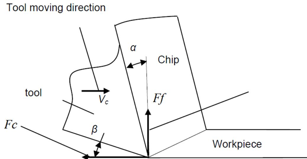
Figure 2-1: Orthogonal cutting forces and angles,  $\alpha$ : rake angle,  $\beta$ : clearance angle,  $F_f$ : feed force,  $F_c$ : cutting force [8]
