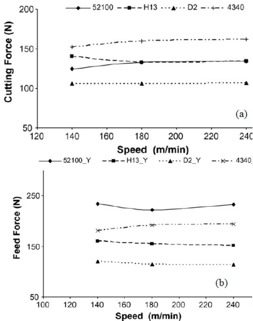
Figure 2-14: (a) Effect of cutting speed and workpiece material on cutting force (b) Effect of cutting speed and workpiece material on feed force [42]
