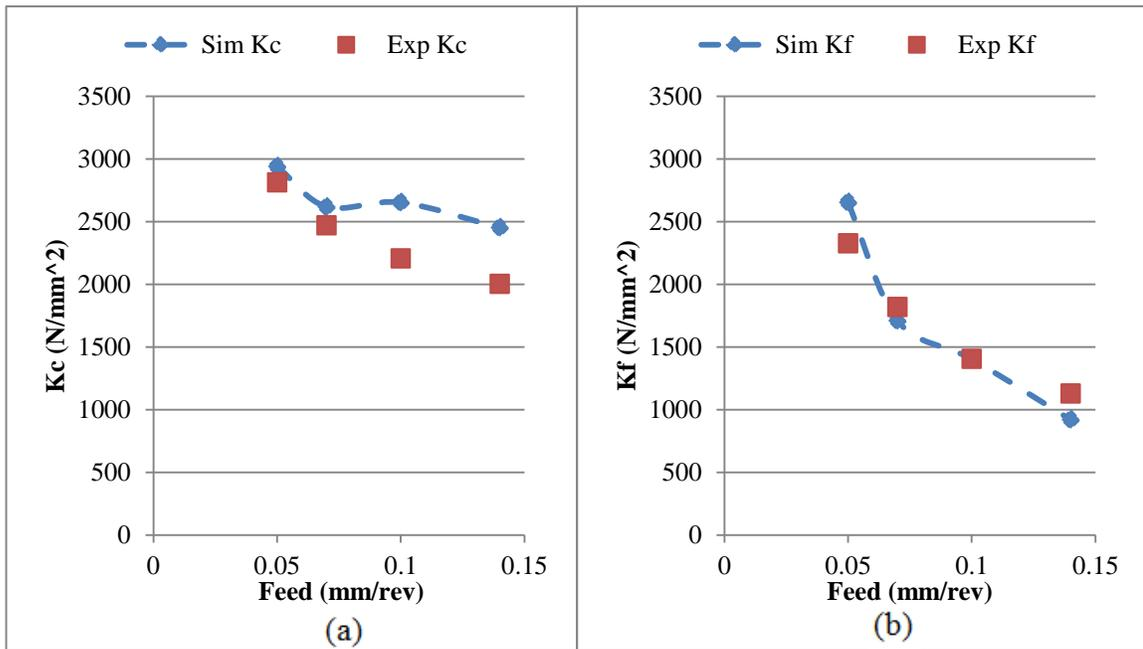
Figure 5-11: Simulation and Experimental results (a) cutting coefficient  $K_c$  (b) cutting coefficient  $K_f$ . Cutting speed  $v=250$  m/min
