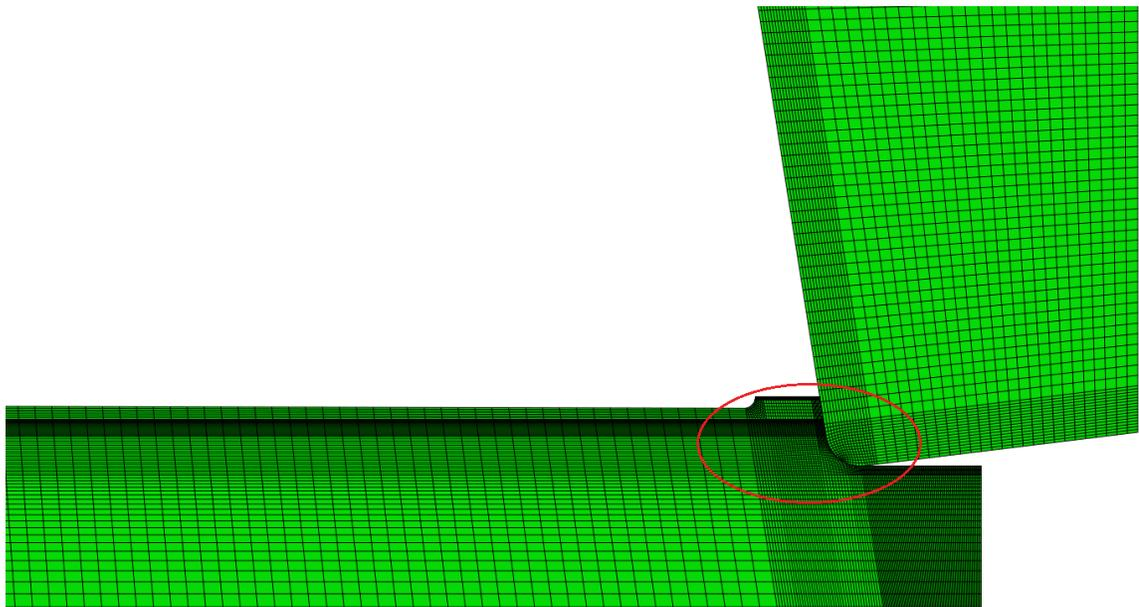
Figure 3-4: Mesh refinement around tool-chip interface and primary and secondary shear zones
