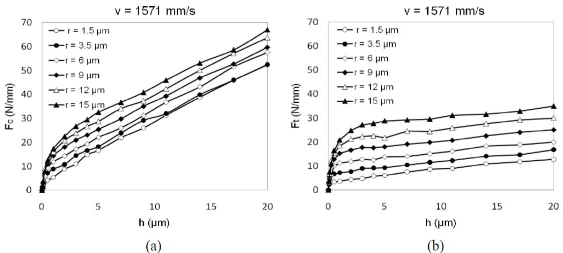
Figure 2-19: FE predicted cutting forces at 1571 mm/s cutting velocity and 3  $\mu\text{m}$  uncut chip thickness in the : (a) cutting direction; (b) feed direction [47]
