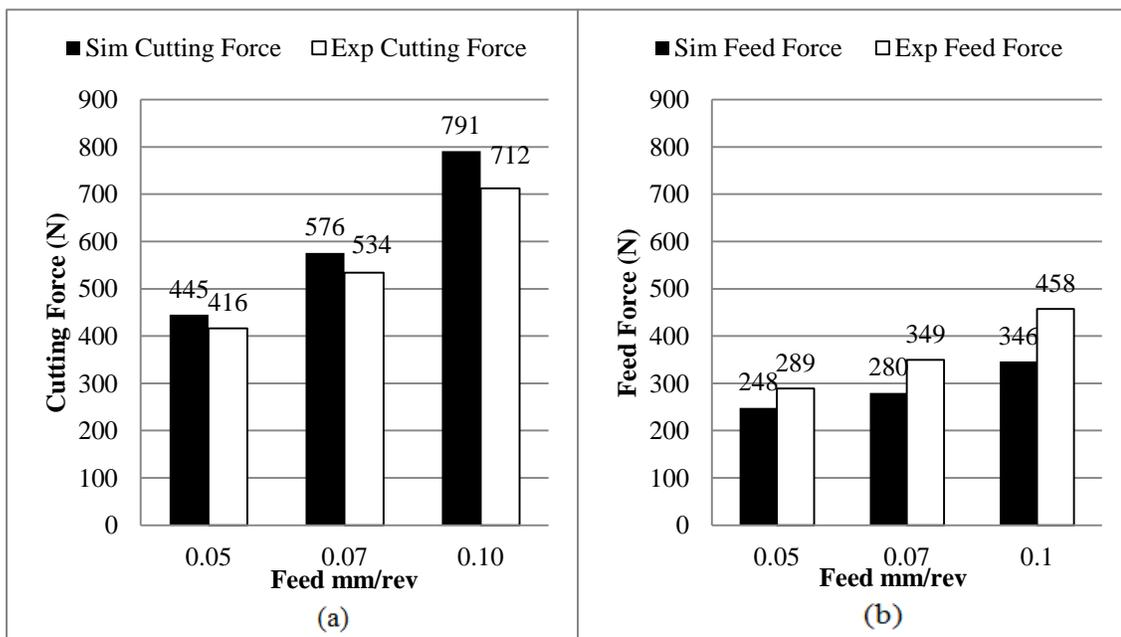
Figure 5-18: Simulation and Experimental results (a) Cutting force  $F_c$  (b) feed force  $F_f$ . Cutting speed  $v=150$  m/min
