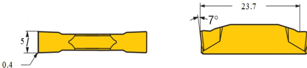
Figure 3-6: A top and front view for the cutting tool- dimensions in mm-(Sandvik Coromant)
