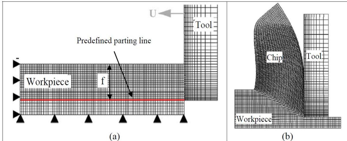
Figure 2-4: Initial boundary condition and geometry when using Lagrangian formulation in FE cutting models. (b) Continuous chip formation using Lagrangian formulation [21]
