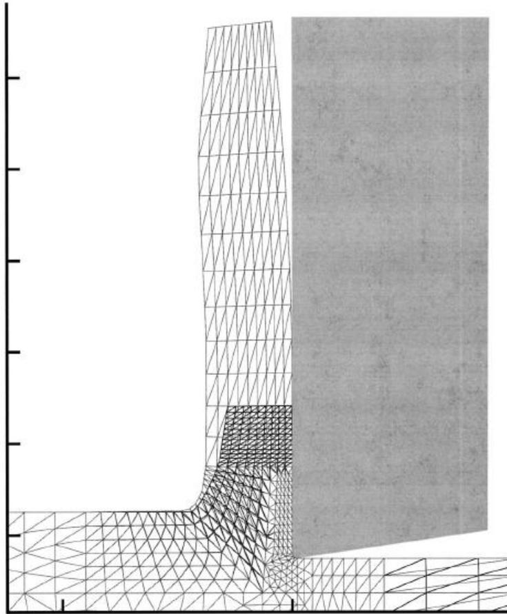
Figure 2-7: Initial and final chip shape in a typical ALE [35]
