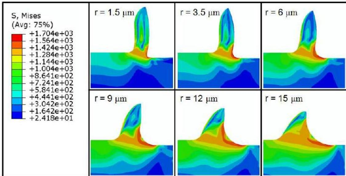
Figure 2-18: Chip morphology and von Mises stresses in MPa for different edge radii obtained at 1571 mm/s cutting velocity, 3  $\mu\text{m}$  uncut chip thickness [47]
