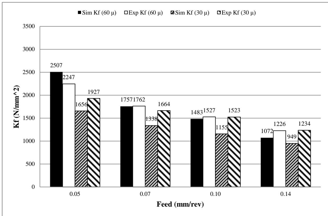
Figure 5-32: Effect of cutting edge radius on  $K_f$  at  $v = 150$  m/min
