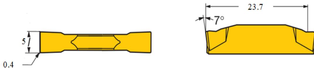
Figure 4-5: A top and front view for the cutting tool-dimensions in mm (Sandvik Coromant)
