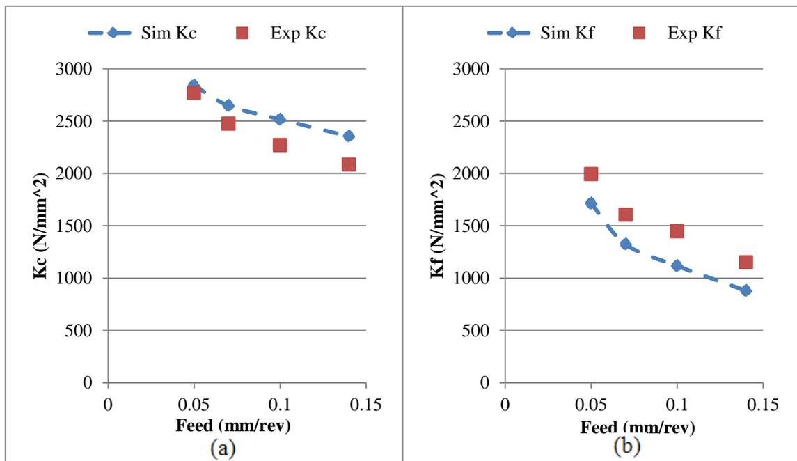
Figure 5-24: Simulation and Experimental results (a) cutting coefficient  $K_c$  (b) cutting coefficient  $K_f$ . cutting speed  $v=200$  m/min
