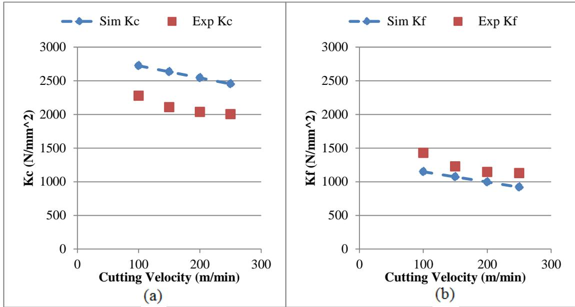
Figure 5-12: Simulation and Experimental results (a) cutting coefficient  $K_c$  (b) cutting coefficient  $K_f$ . Feed rate  $f=0.14$  mm/rev
