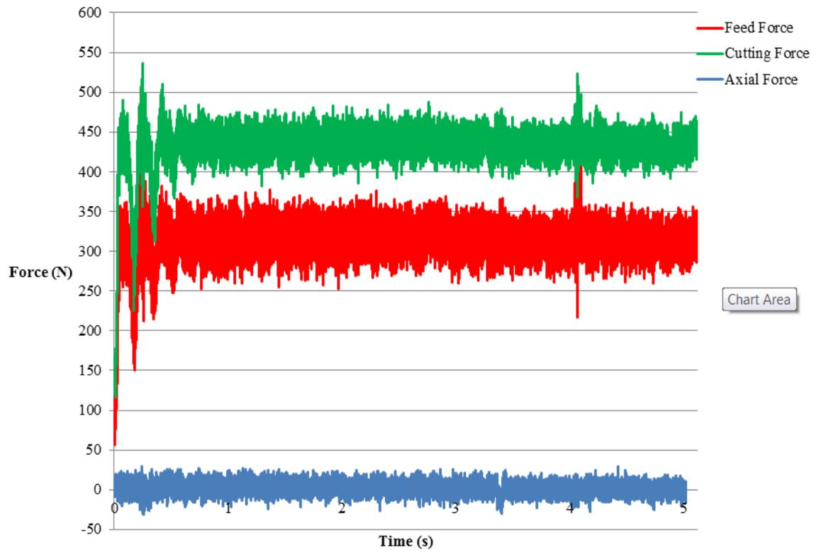
Figure 4-11: Example of forces obtained experimentally at  $f=0.05$  mm/rev,  $v=100$  m/min
