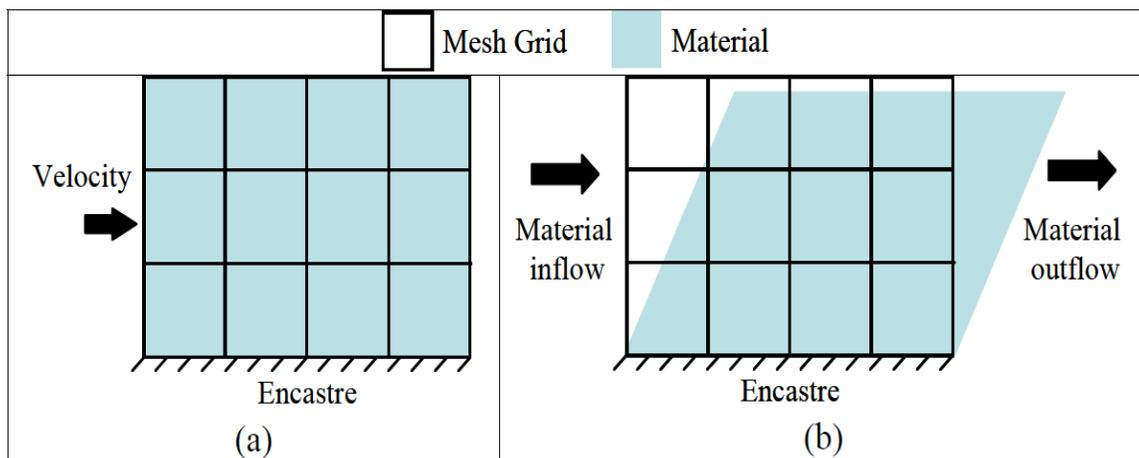
Figure 2-5: Initial position of mesh grids and material. (b) Final position of mesh grid and material flow when using Eulerian formulation [9]
