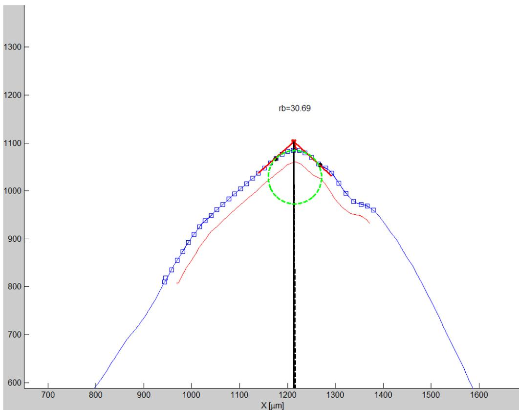
Figure 4-7: MATLAB graph for calculating the cutting edge radius
