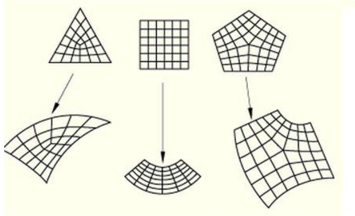
Figure 3-2: Structured Mesh [48]
