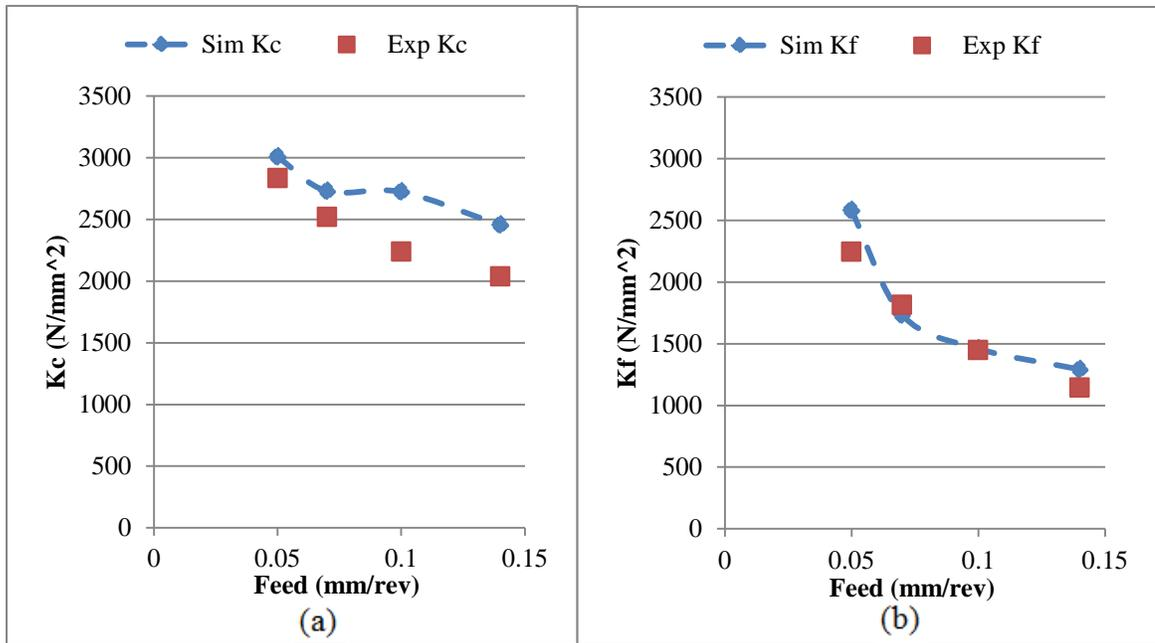
Figure 5-10: Simulation and Experimental results (a) cutting coefficient  $K_c$  (b) cutting coefficient  $K_f$ . Cutting speed  $v=200$  m/min
