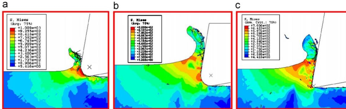
Figure 2-11: Size effect at different uncut chip thickness. (a)  $h = 1 \mu\text{m}$ ; (b)  $h = 4 \mu\text{m}$  (c)  $h = 20 \mu\text{m}$ . [5]
