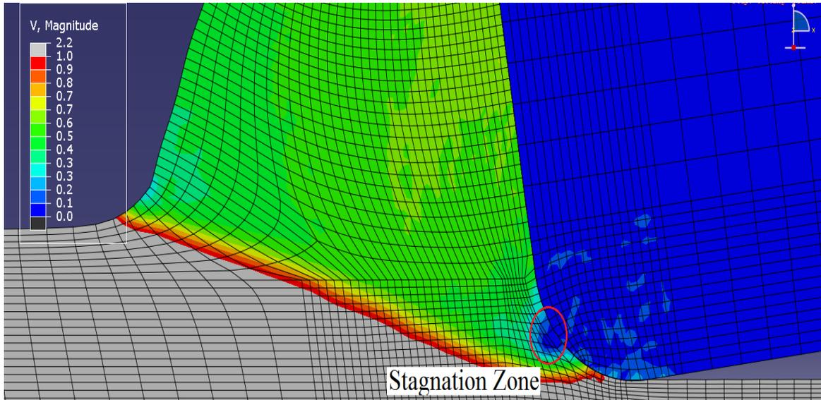
Figure 5-27: stagnation zone at cutting radii  $\rho_e = 60 \mu\text{m}$  cutting speed  $v = 100 \text{ m/min}$  feed rate  $f = 0.05 \text{ mm/rev}$
