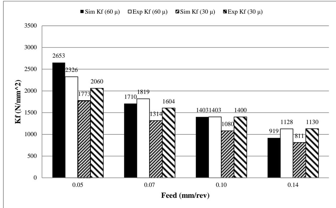
Figure 5-36: Effect of cutting edge radius on  $K_f$  at  $v = 250$  m/min
