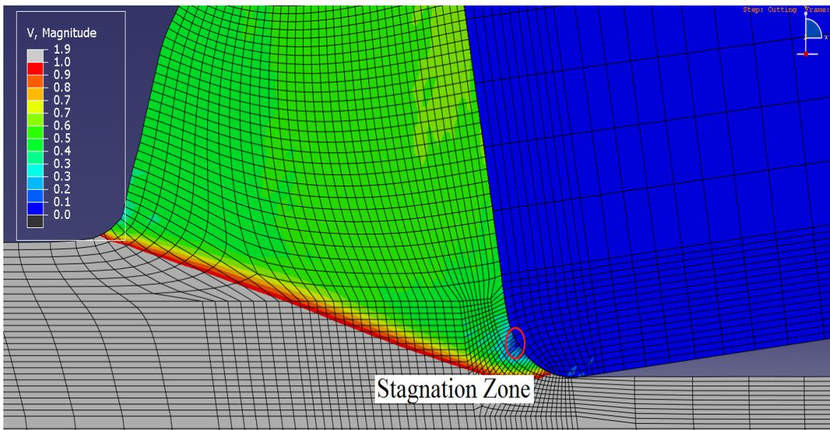
Figure 5-28: stagnation zone at cutting radii  $\rho_e = 30 \mu\text{m}$  cutting speed  $v = 100 \text{ m/min}$  feed rate  $f = 0.05 \text{ mm/rev}$
