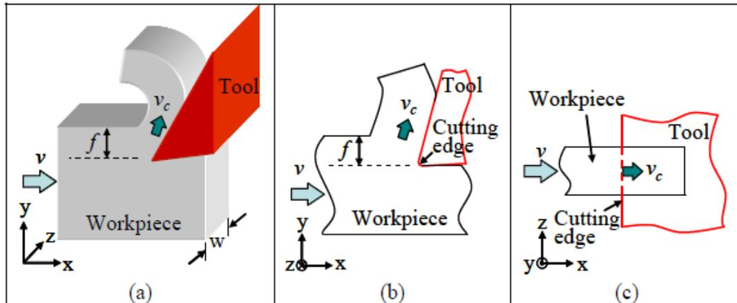
Figure 2-2: Orthogonal machining process. (a) 3-dimensional view. (b) Front view. (c) Top view. [9]
