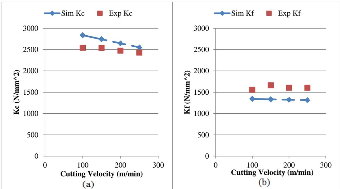
Figure 5-22: Simulation and Experimental results (a) cutting coefficient  $K_c$  (b) cutting coefficient  $K_f$ . Feed rate  $f = 0.07$  mm/rev
