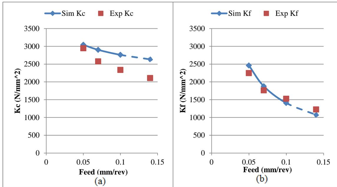
Figure 5-6: Simulation and Experimental results (a) cutting coefficient  $K_c$  (b) cutting coefficient  $K_f$ . Cutting speed  $v=150$  m/min
