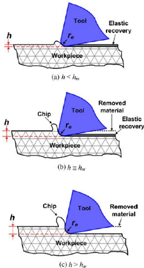
Figure 2-9: Chip formation relative to the minimum chip thickness in micro-scale machining [39]
