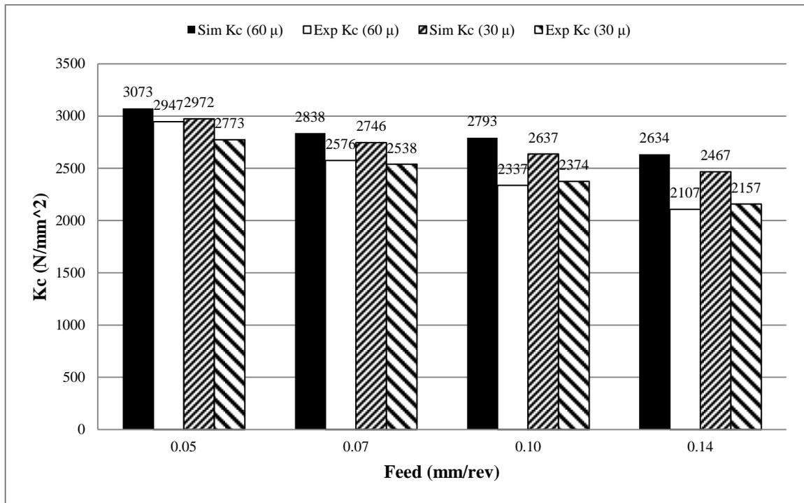
Figure 5-31: Effect of cutting edge radius on  $K_c$  at  $v = 150$  m/min
