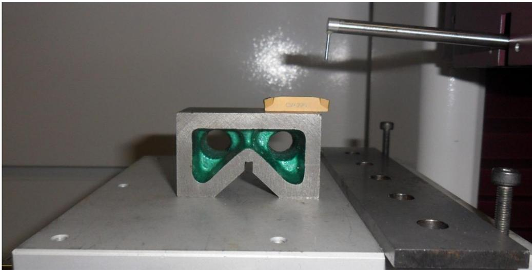
Figure 4-6: Mitutoyo Formtracer for measuring the tool cutting edge radius
