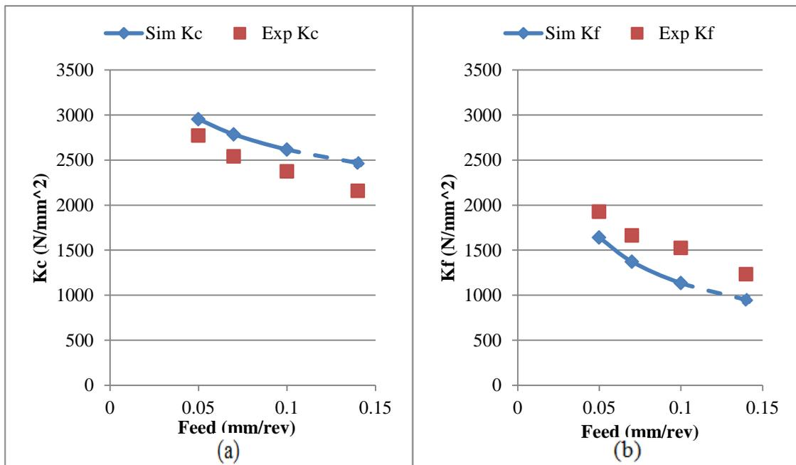
Figure 5-20: Simulation and Experimental results (a) cutting coefficient  $K_c$  (b) cutting coefficient  $K_f$ . cutting speed  $v=150$  m/min
