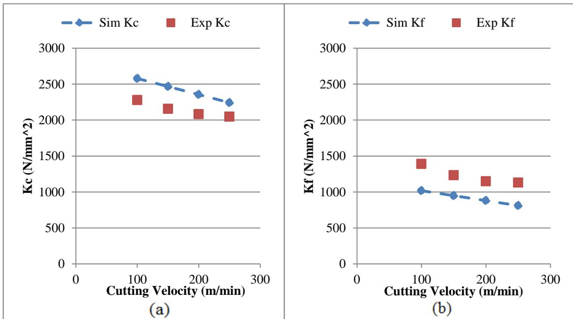
Figure 5-26: Simulation and Experimental results (a) cutting coefficient  $K_c$  (b) cutting coefficient  $K_f$ . Feed rate  $f=0.14$  mm/rev
