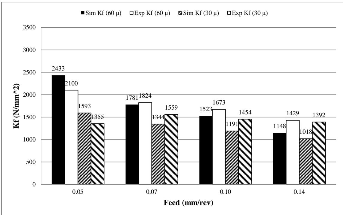
Figure 5-30: Effect of cutting edge radius on  $K_c$  at  $v=100$  m/min
