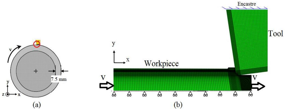
Figure 3-8: (a) Portion of experiment set up being modeled. (b) B.C. for FE cutting model
