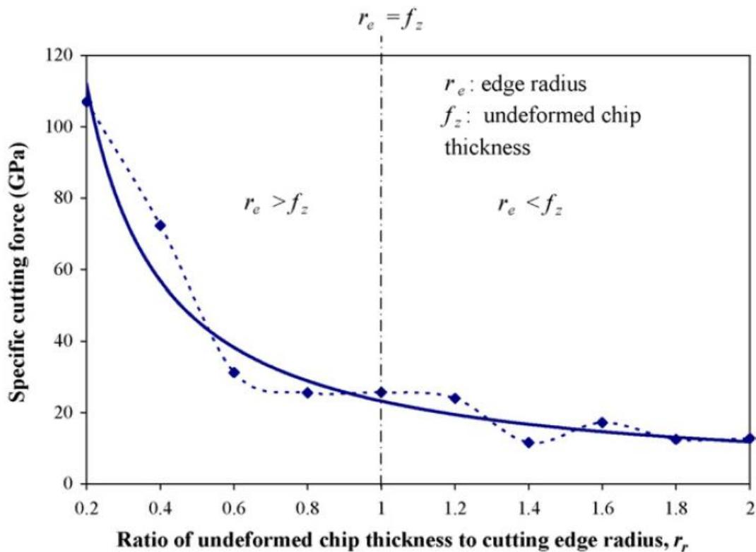
Figure 2-10: Specific cutting force in feed direction [39]
