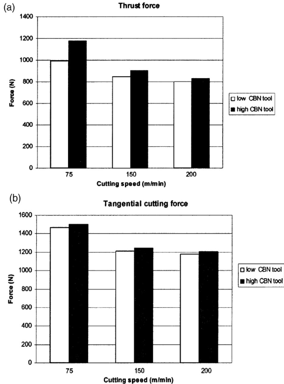
Figure 2-15: The predicted cutting forces when using different CBN content tools: (a) thrust force with cutting speed 75, 150, and 200 m/min; (b) tangential cutting force with cutting speed 75, 150, and 200 m/min. [43]
