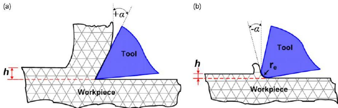
Figure 2-17: cutting edge in (a) macro-scale and (b) micro-scale cutting. [39]
