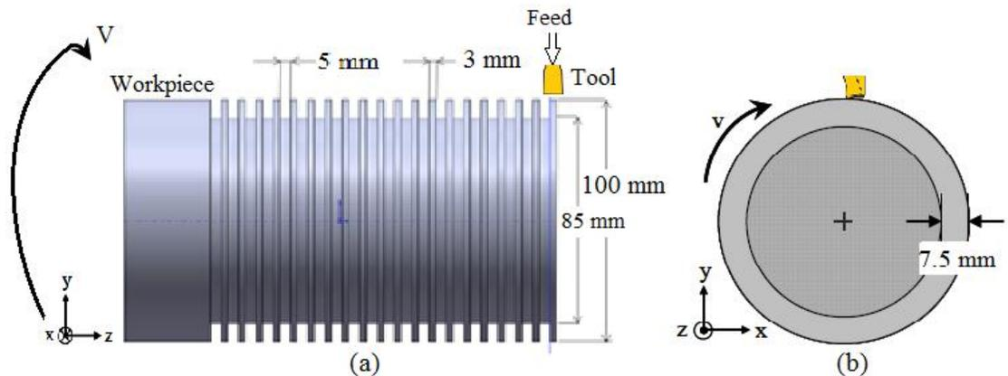
Figure 3-7: The experiment set up for plunging process. (a) Front view (b) Side view
