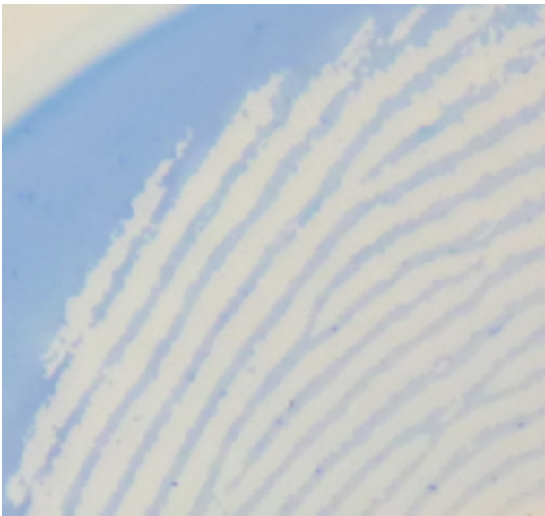
Figure 4.2 A contrasted image of a partial fingerprint captured on PES membrane. Details such as bifurcation are seen clearly. Positive pattern transfer.
