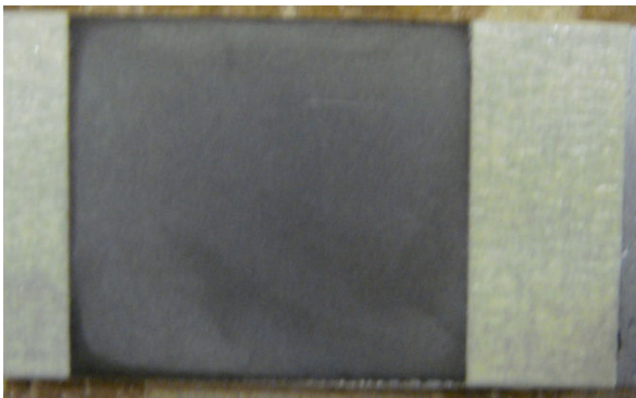
Figure 5-20: Manganese deposited on Cu with \text{NH}_2\text{OH}\cdot\text{HCl} .
