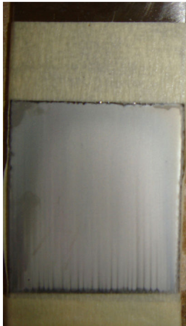
Figure 5-14: Smooth metallic cobalt coating obtained from a pH 2.30 solution.
