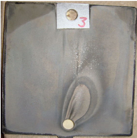
Figure 5-16: Edge effects at lower hole when Mn was plated at 70 \text{ mA}\cdot\text{cm}^{-2} on cobalt coated chromium.
