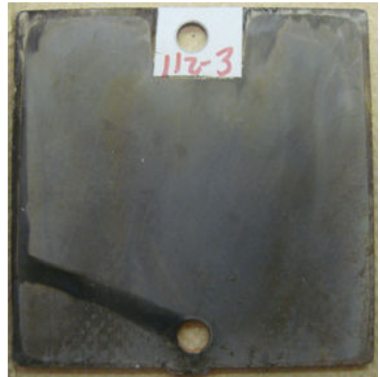
Figure 5-5: Mn plated on 100 cm 2 cobalt-coated sample with Cu interlayer.
