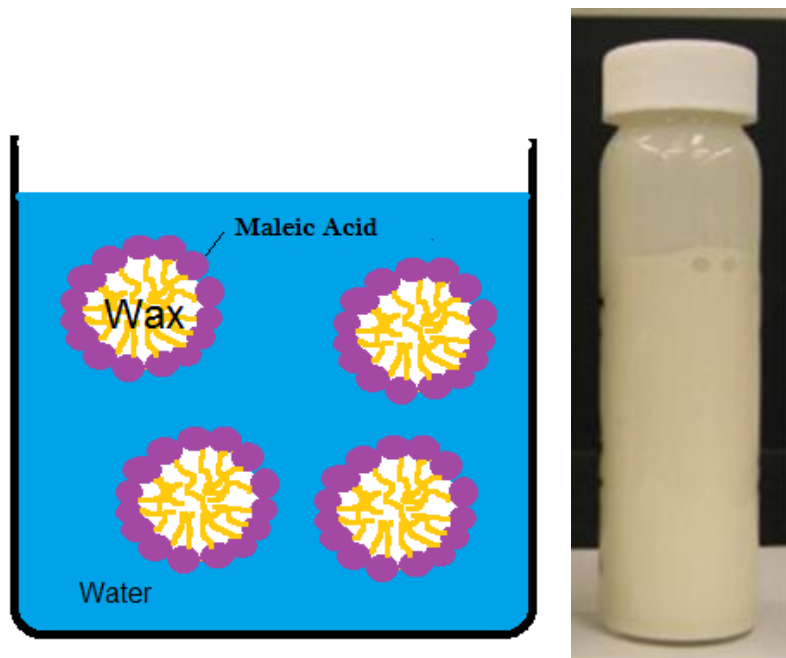
Figure 8 (Left)-Theoretical Cross Section of Wax Emulsion (Right)-Photo of Wax Emulsion
