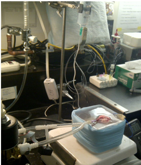
Figure 3.2. Image of rodent ventilator model. The lungs were suspended in PBS held at 37^{\circ}\text{C} . The pulmonary artery was perfused with Krebs + BSA buffer held 30 cm above the tissue.
