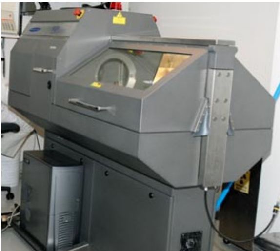
Figure 5.0. X-SPECT small animal scanner (Gamma-Medica, Inc.). This scanner performed all micro-CT assessments of rat lung density during lung fibrogenesis. Image taken from www.gammamedica.com .
