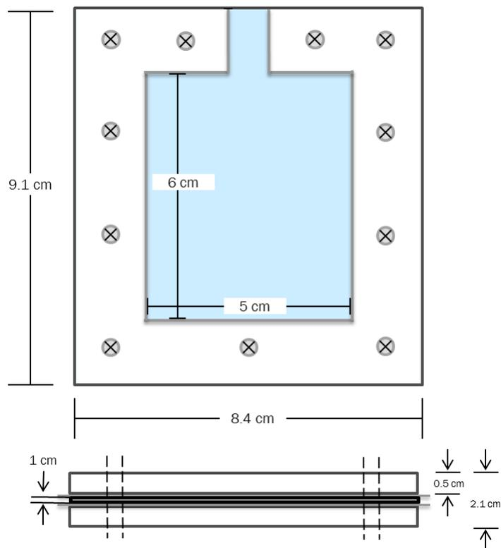
**Figure 4.2:** Schematic diagram of the mold used for the polymerization of silicone hydrogel materials in the current research.
