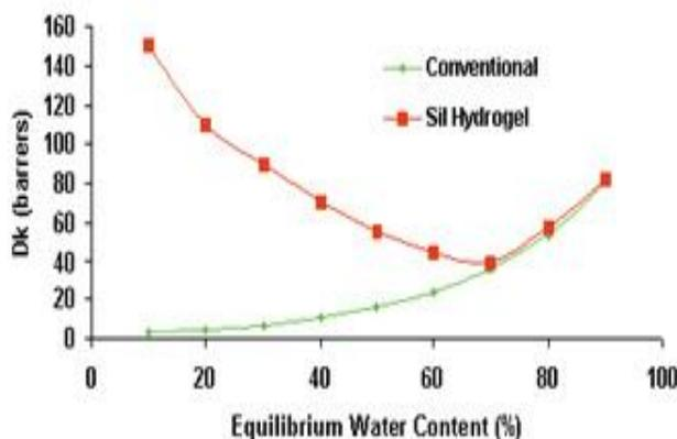
**Figure 2.1:** Relationship between Oxygen Permeability and Equilibrium Water Content of commercially available silicone and conventional contact lenses (Jones, 2002).
