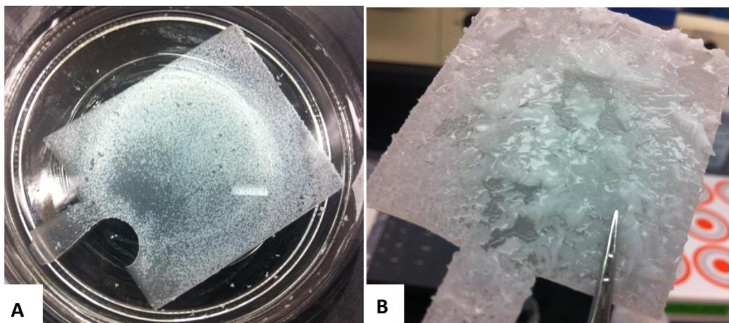
**Figure 5.1:** PVP-containing DMA/TRIS hydrogel discs immersed in milliQ water A. 2wt% PVP (10 kDa) and B. 5 wt% PVP (10 kDa) was incorporated during synthesis. Incompatibility between the hydrophilic phase DMA and the wetting agent PVP created a layer on the materials surface that peeled off upon hydration.
