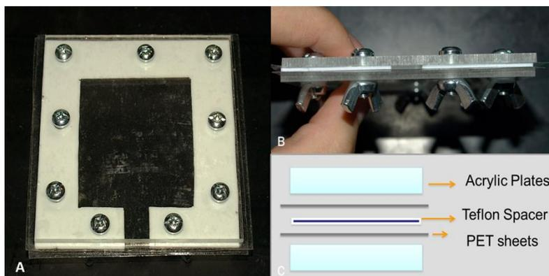
**Figure 4.1:** (A, B) Acrylic mold used for the preparation of silicone hydrogels, (C) Schematic representation of the acrylic mold components.
