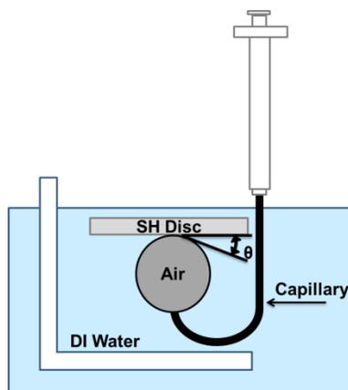
**Figure 4.3:** Schematic illustration of captive bubble technique used for contact angle measurements of the surface for silicone hydrogels.
