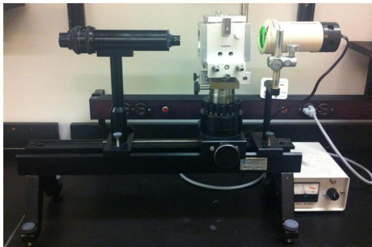
**Figure 4.4:** Goniometer apparatus (Ramé-Hart NRL 100-00 Contact Angle Goniometer) used for the measurement of the contact angle.
