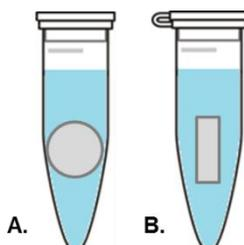
**Figure 4.5:** Schematic illustration of the silicone hydrogel disc placed in the eppendorf tubes with 1 ml PBS for the release study.
