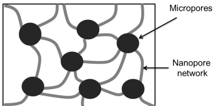
**Figure 2.2:** Schematic illustration of possible nanopore and micropore interconnected structure of silicone hydrogel contact lens materials.
