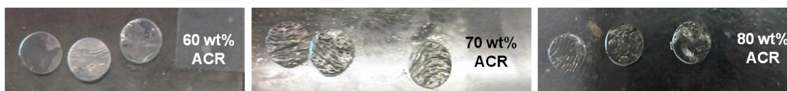
Figure 5: Copolymer coupons obtained using a 0.635 mm punching tool once the solid elastomers had been synthesized, soaked in propanol for 12 h and dried for 48 h.
