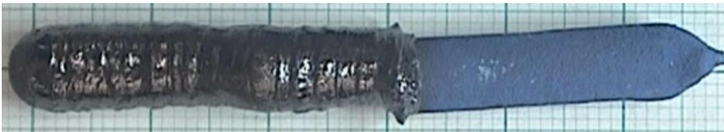
Figure 2.5: Result of a Pre-melt of Cobalt Niobate
