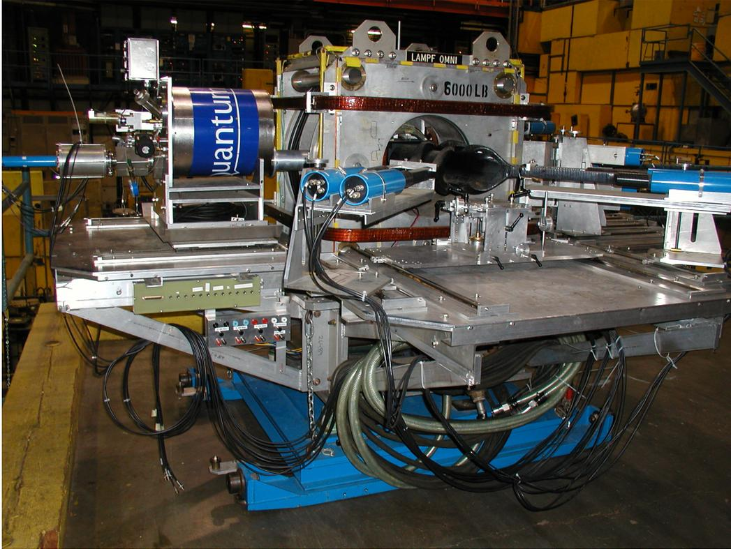
Figure 5.1: The OMNI-LAMPF Instrument Fit with Gas Flow Cryostat (Image Courtesy of TRIUMF)
