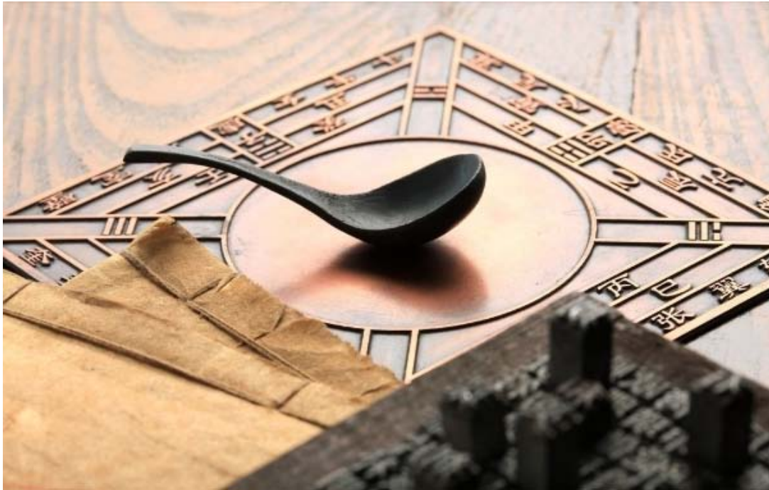
Figure 1.1 Model of the first instrument known to be a compass, called SiNan [2].
