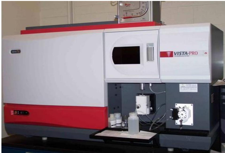
Figure 33: ICP-OES apparatus used in the MSE department at McMaster University
