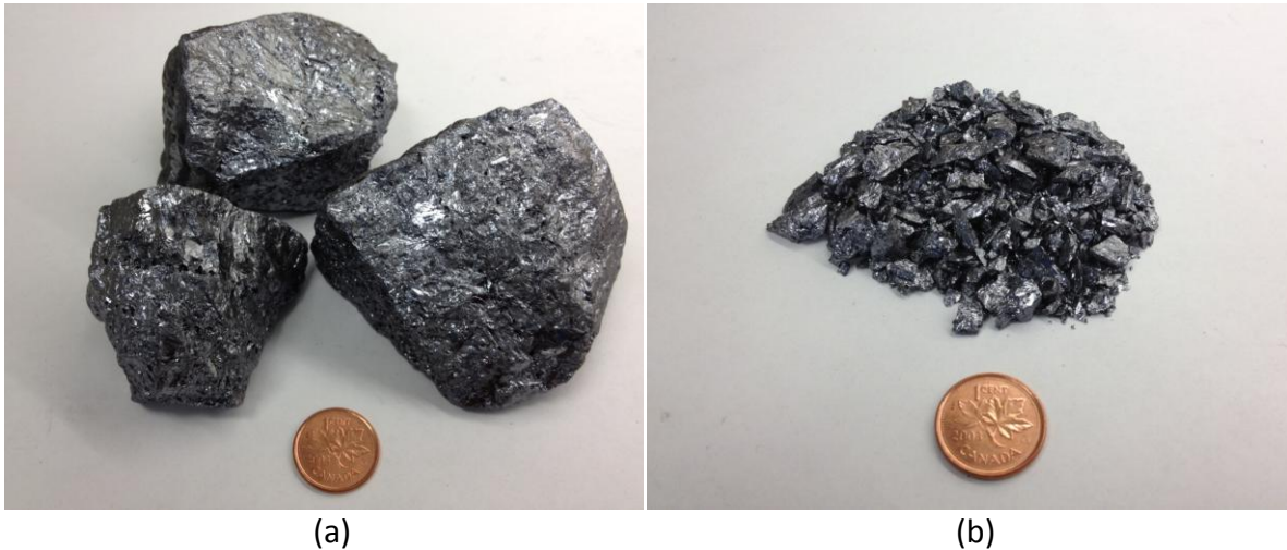
Figure 27: MG silicon used for the experiments (a) as received (b) crushed
