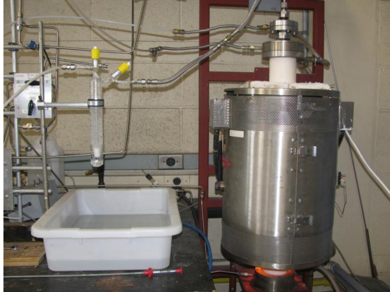
Figure 29: Tube furnace used for the experiments
