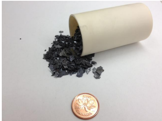
Figure 28: High alumina crucible used for the experiments
