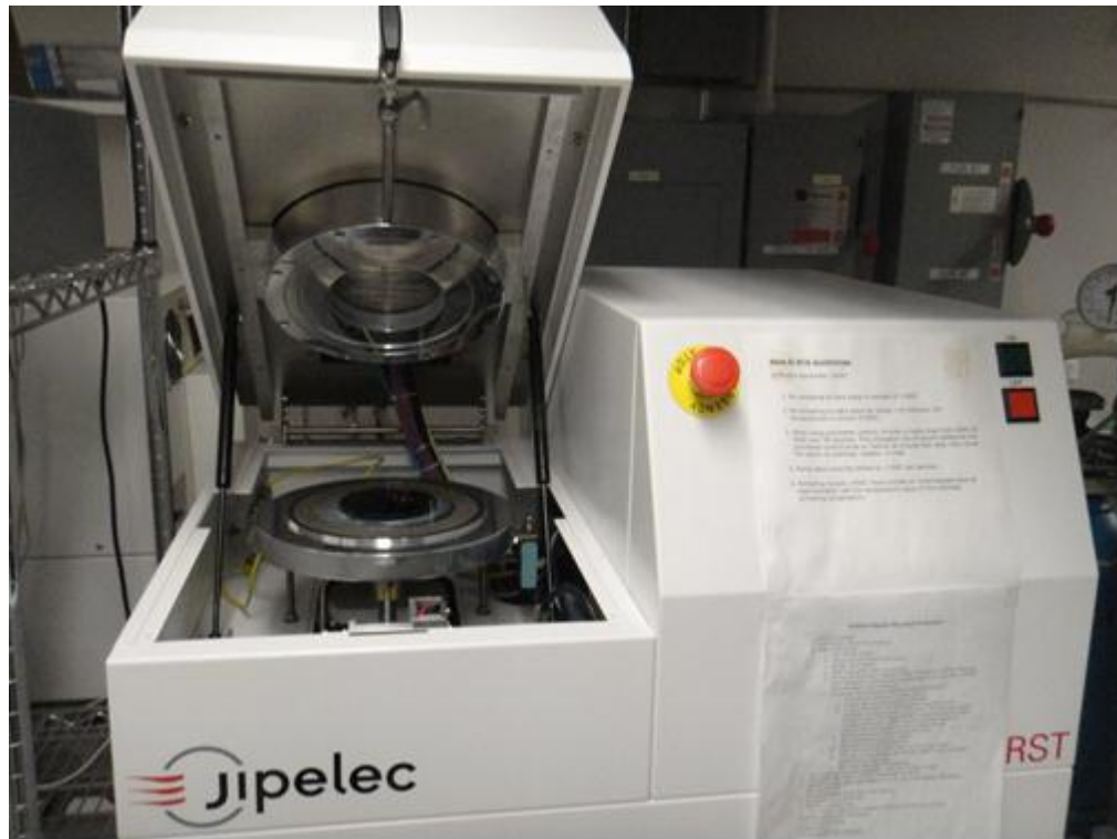
Figure 36: Sample chamber of the RTP of McMaster University.
