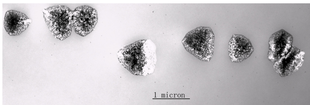
Figure 2.5 TEM of the organosiloxane gel after 7 days of irradiation. Samples for microscopy were prepared by redispersing the gel in iso -propanol and casting the colloid onto Cu grids.
