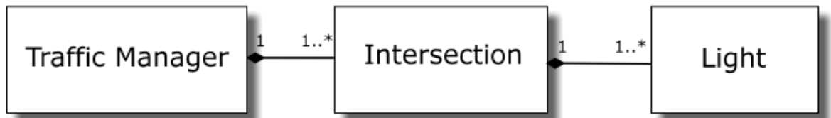
Figure 4.5: A uml description of traffic system. Traffic Manager is composed of Intersections and Intersections are composed of Lights.
