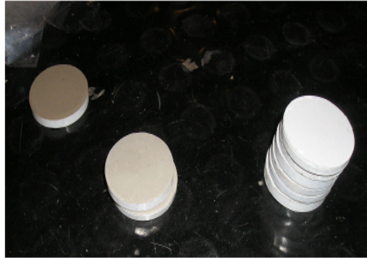
Figure 4-7. Slag analysis: compact pellet of mill slag.
