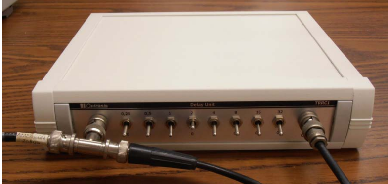
Fig. 6.4: Optronics-TRRC1 as the delay generator for generating stop signals
