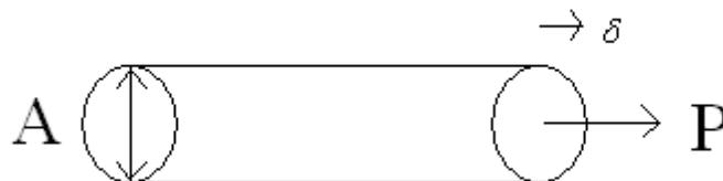
Figure 2.01: Schematic diagram of a rod subjected to a uniform axial load  $P$  over a cross section of area  $A$ , with elongation  $\delta$ .
