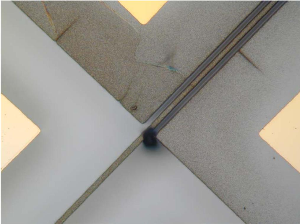
Figure 4.15: View of a sample fabricated by the backside etch process with flip procedure, showing a bridge running between the electrodes. Burn marks can be seen.
