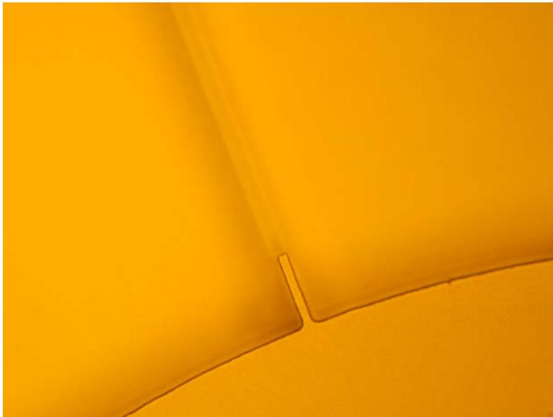
Figure 4.19: A third view of the same sample, showing a missing bridge
