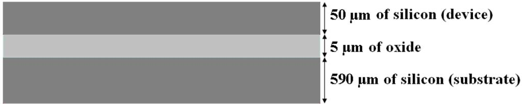
Figure 4.01: Side view of SOI wafer (not to scale)
