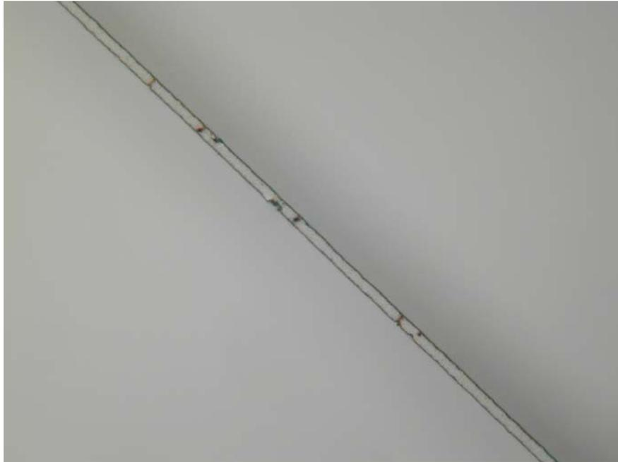
Figure 4.16: Another view of the same sample. Burn marks and cracks on a bridge can be seen.
