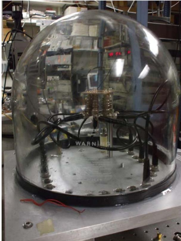
Figure 5.08: Device in vacuum, achieved by using a bell jar and a pump
